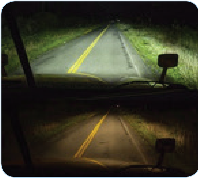
In snowplow headlights, using LED bulbs (top) instead of halogen bulbs (bottom) can improve visibility by allowing operators to more easily see objects at greater distances.
