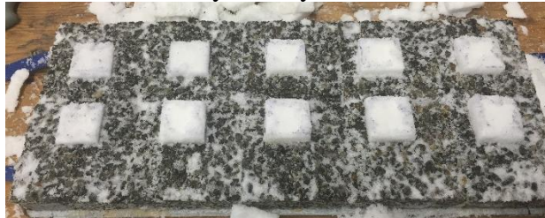
OGFCma5y Dry Salt test
