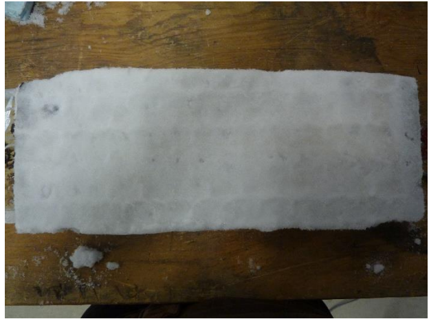
Figure 12: UTFC-ny sample during a deicing test with dry salt before and after trafficking.
