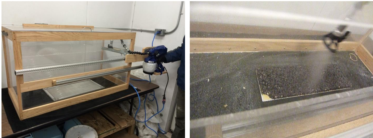
Figure 8: Enclosure and sprayer for anti-icing pavements.
