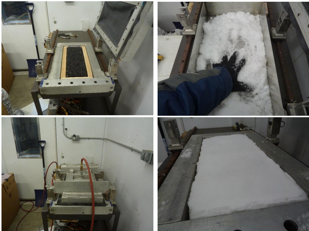
Figure 7: Snow application and compaction sequence (top left: pavement sample in compaction box; top right: snow being re-sieved; bottom left: lid closed during compaction; bottom right: compacted snow).
