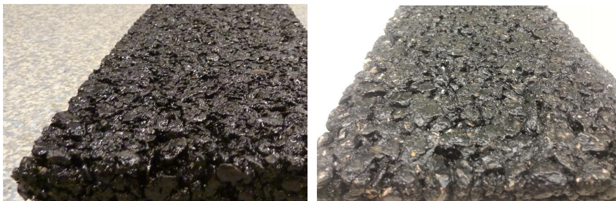
Figure 3: Ultrathin friction course pavements made with pavement mix from New York with \frac{1}{2} inch max aggregate (left) and Missouri with \frac{3}{4} inch max aggregate (right).
