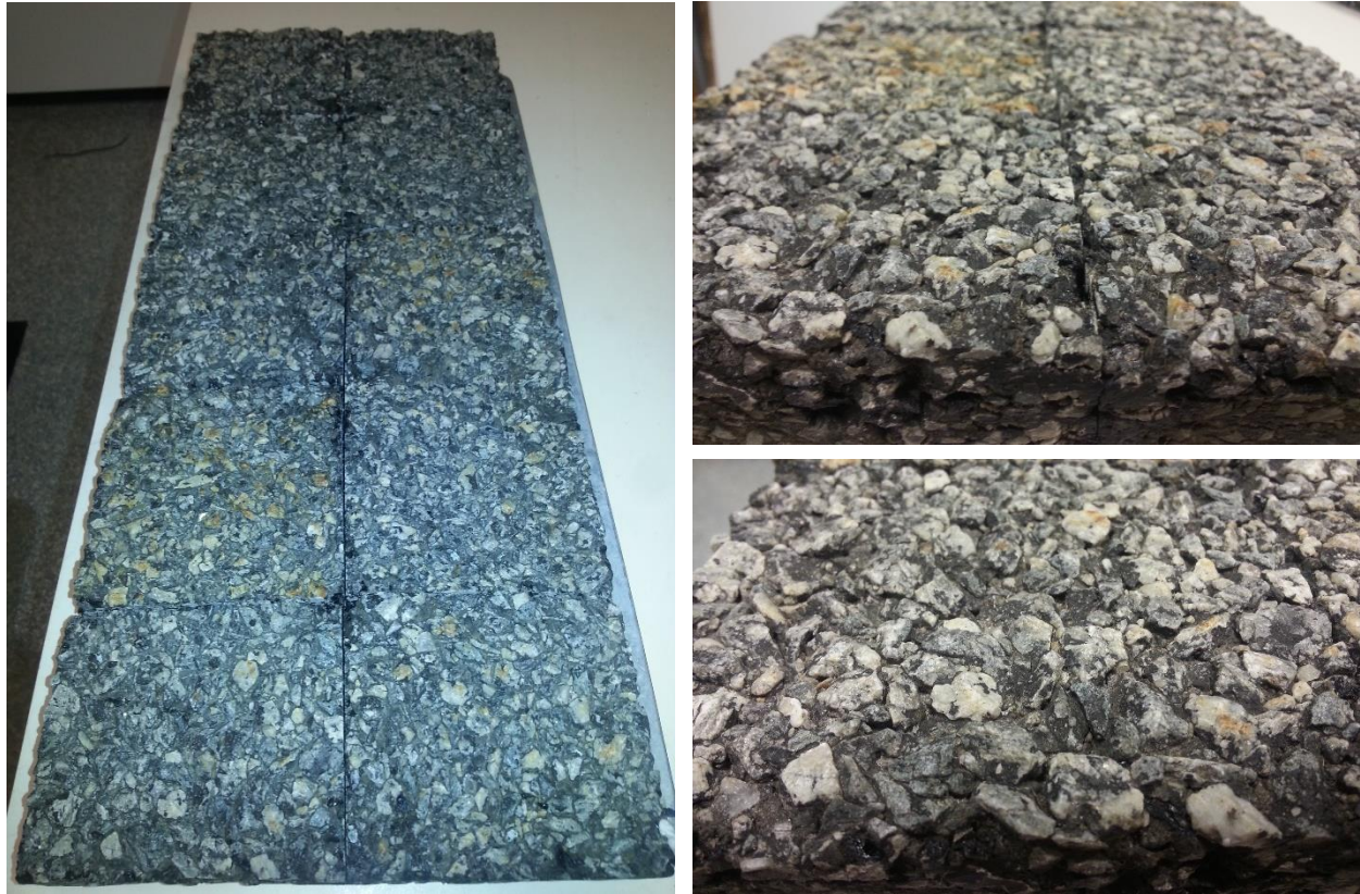
Figure 5: Open-graded friction course pavement from Massachusetts cores (OGFC-ma5y).
