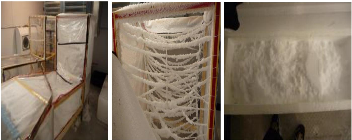
Figure 6: Snow making process and snow storage.
