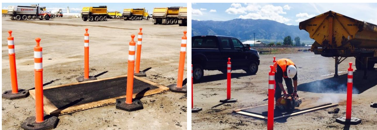
Figure 1: DGP compacted in wood form (left) and cutting samples (right).
