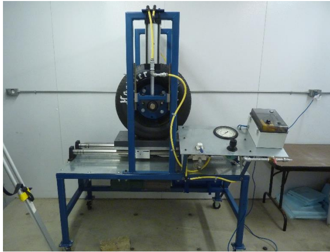
Figure 11: Simulated trafficking device.
