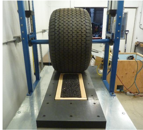
Figure 11: Simulated trafficking device.
