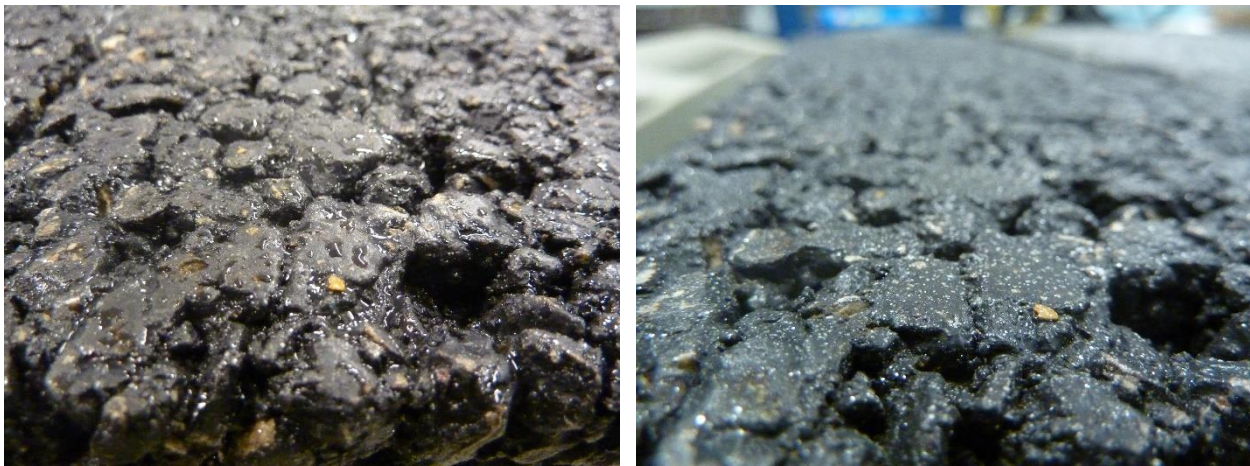
Figure 9: Close-up of a pavement sample after applying salt brine (left) and after drying (right).
