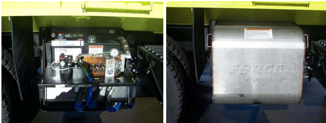
Figure 104. The various components enclosed in the valve body box are expensive and critical to the operation (left), the use of a sealed stainless steel enclosure will help prolong the life of these components (right) (Mills, 2012).
