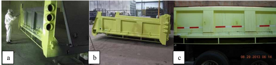
Figure 55. a & b) A new body treated with PRP CORSOL, then top coated with PRP Acrylic Urethane, c) a dump body after 5 years of use on a salt spreader truck (WSDOT & PRP, 2014).
