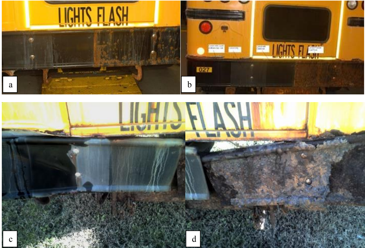
Figure 59. a) 60 APG cycles, b) 100 APG cycles, c & d) 150 APG cycles of Corsol system compared (left) to standard powder coat (right) (PRP, 2014).
