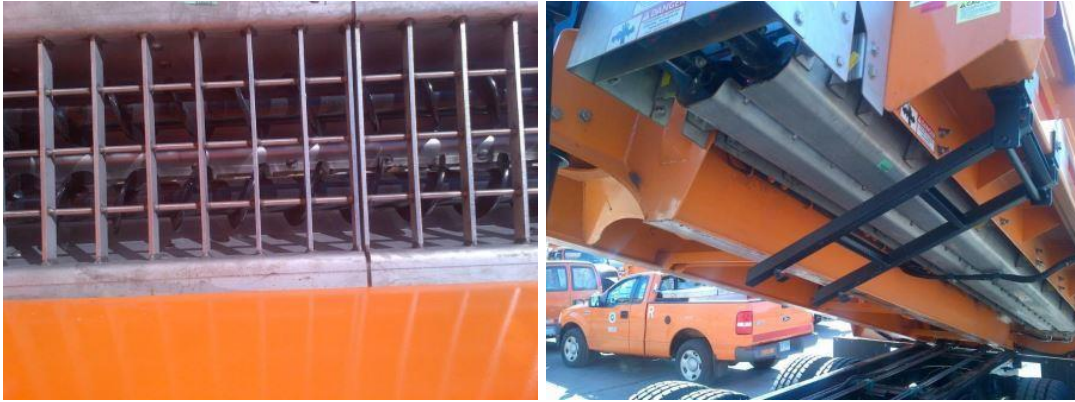
Figure 52. ConnDOT auger system tray that bolts into the current sanding chain area of the body (Chupas, 2014).
