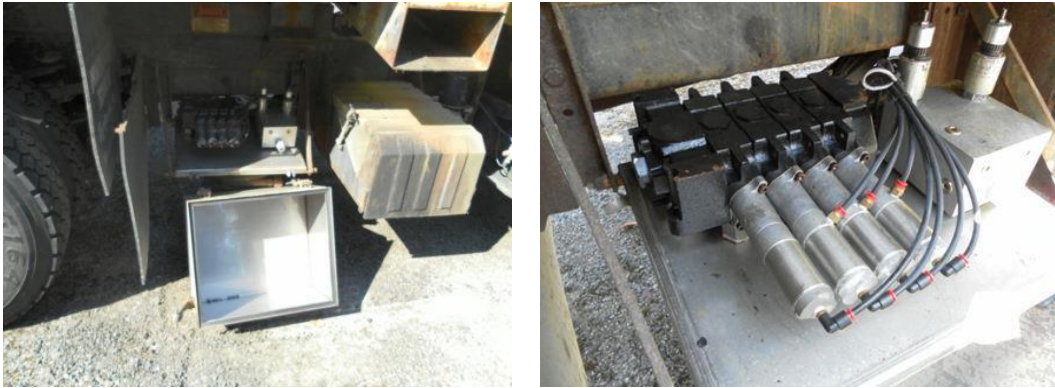
Figure 96. Hydraulic components protected from corrosion using modified sealed protective covers (Shi et al., 2013).
