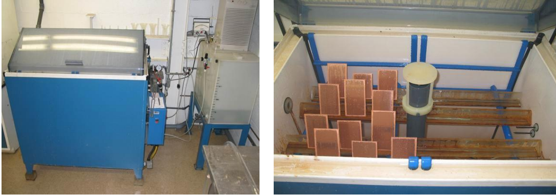
Figure 63. ASTM B117 test chamber and specimens as loaded into the salt spray (Shi et al., 2013).
