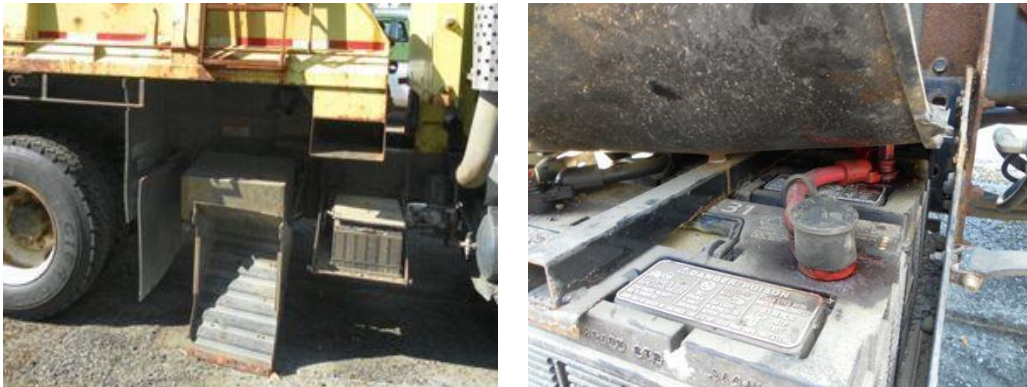
Figure 97. Modified protective cover for a battery to reduce harmful effects of corrosion (left), and rubber caps on battery terminals used to mitigate effects of corrosion (right) (Shi et al., 2013).
