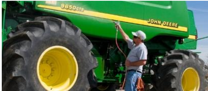
Figure 50. Fluid Film applied to frame rails and undercarriage (Chupas, 2014; Fluid Film, 2014).
