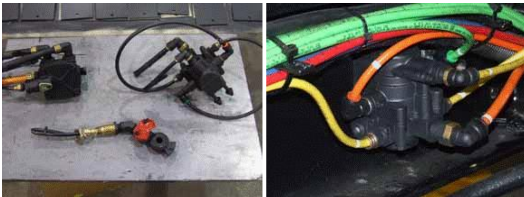
Figure 56. Brake valves and glad hand treated with CORSOL prior to installation (WSDOT & PRP, 2014).
