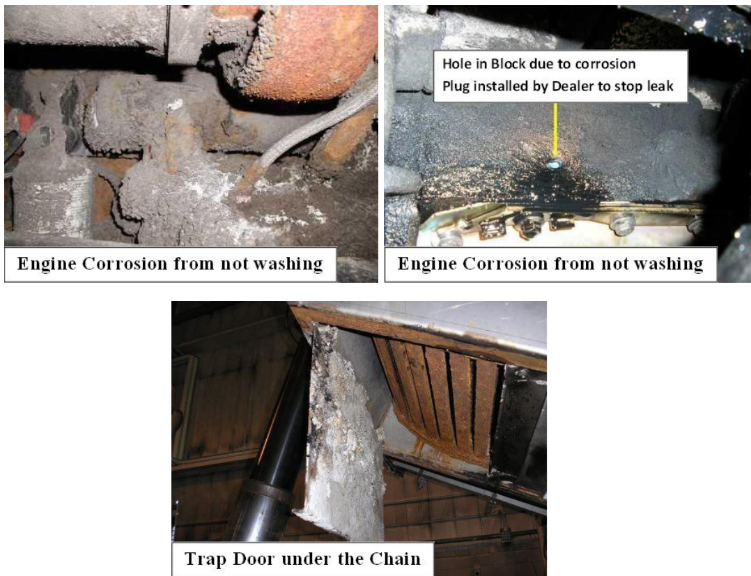
Figure 22. Images of corrosion damage on NYSDOT vehicles (courtesy of NYSDOT).
