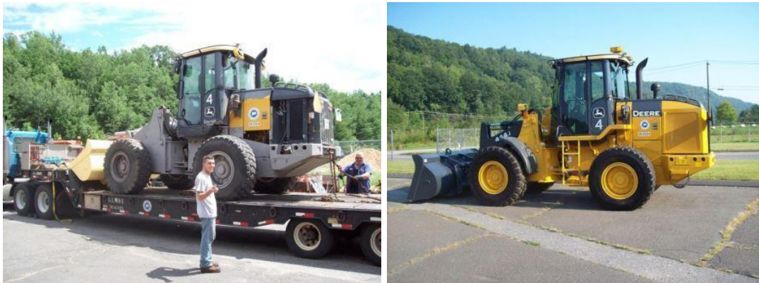
Figure 39. A vehicle which first sandblasted (left) and then primed and painted (right) (Chupas, 2014).
