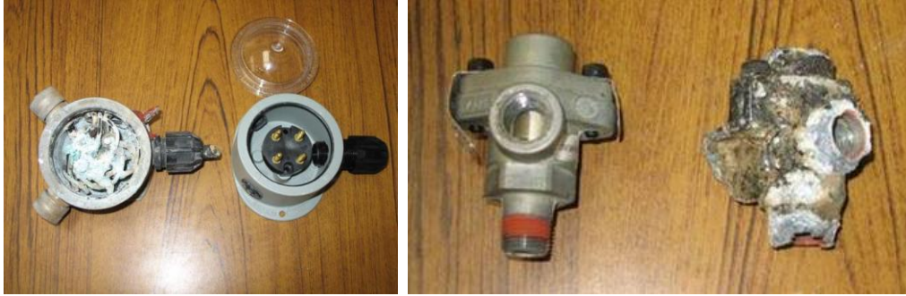
Figure 18. Image of salt-related vehicle damage (Mills, 2011 and 2012).
