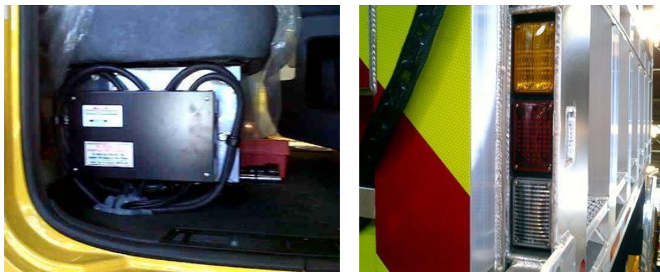
Figure 46. New lighting control module under the passenger seat (left), newly adopted lighting package (right) (Smith, 2014).
