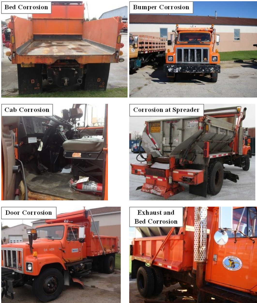
Figure 21. Images of corrosion damage on (Michigan DOT vehicles courtesy of MDOT).
