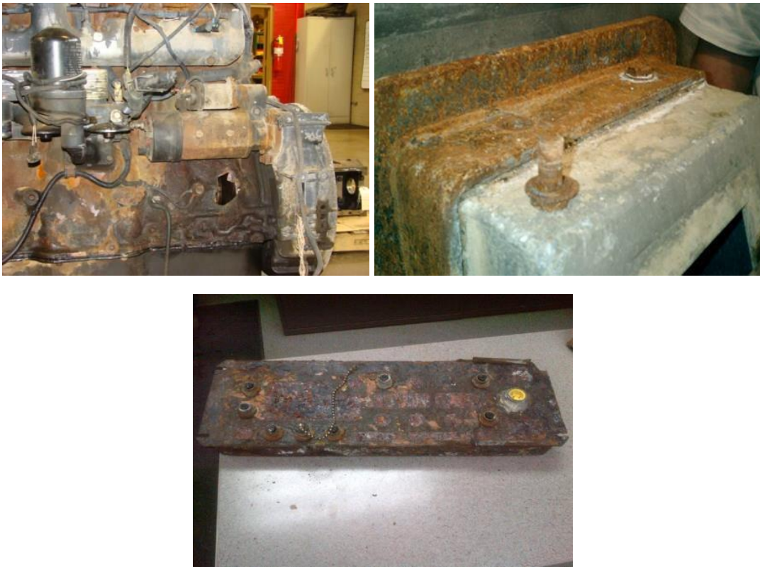
Figure 19. Images of corrosion damages on PennDOT vehicles (Smith, 2014).
