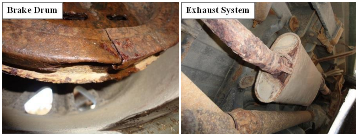
Figure 17. Images of salt-related damage on brake drum and exhaust system (Shi, 2014).
