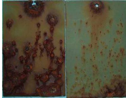
Figure 90. Accelerated corrosion testing (Koch, 2011).
