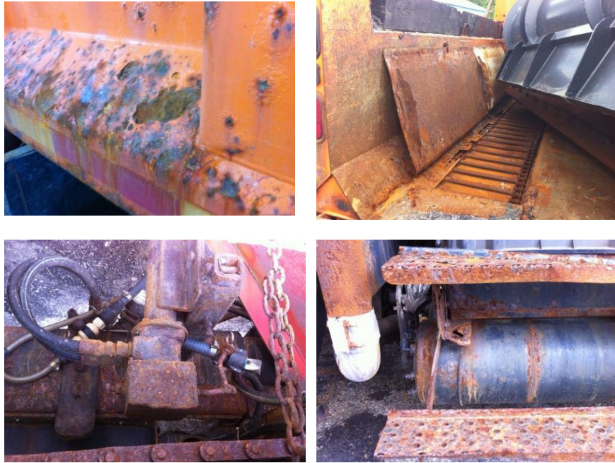
Figure 26. Images of damages due to corrosion on VAOT vehicles (courtesy of VAOT).
