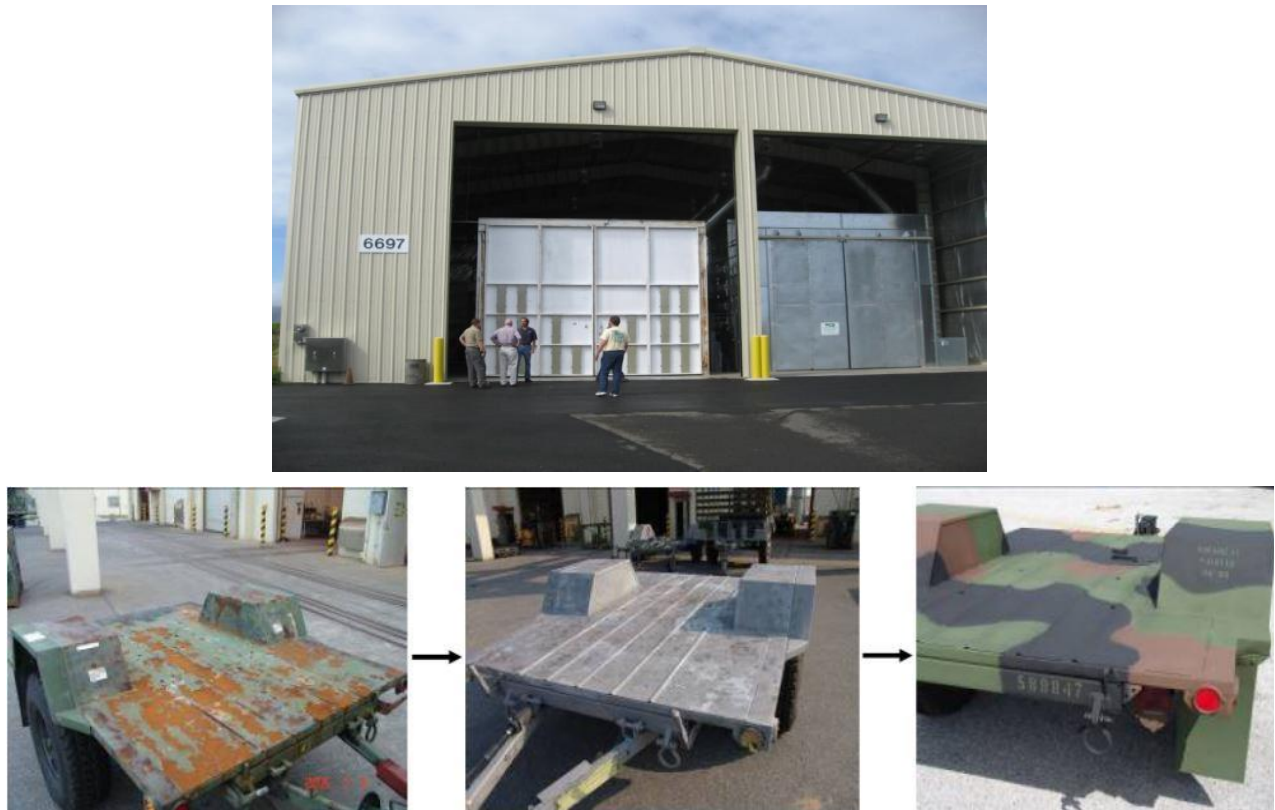
Figure 86. Fixed corrosion repair facilities (Koch and Friend, 2009).
