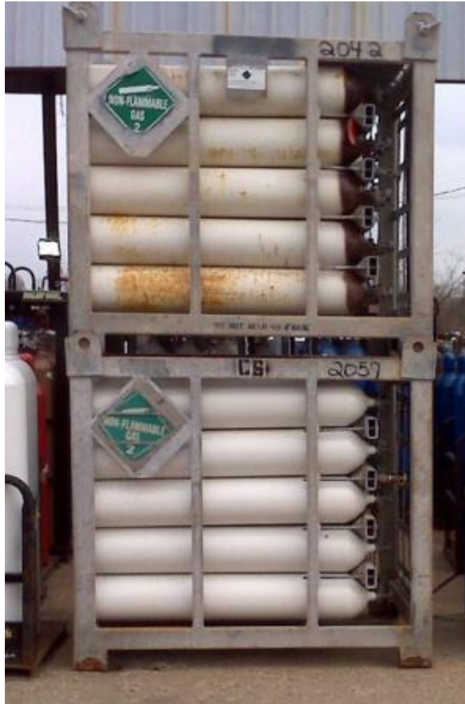
Figure 60. The standard cylinder group on top compared to the PRP treated cylinders on the bottom (PRP, 2014).
