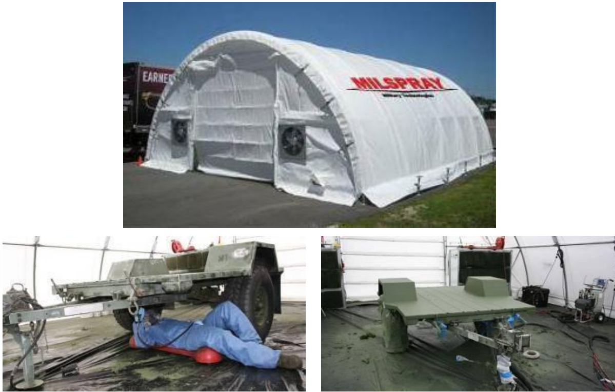
Figure 87. Mobile corrosion repair facilities (Koch and Friend, 2009; Koch, 2010).
