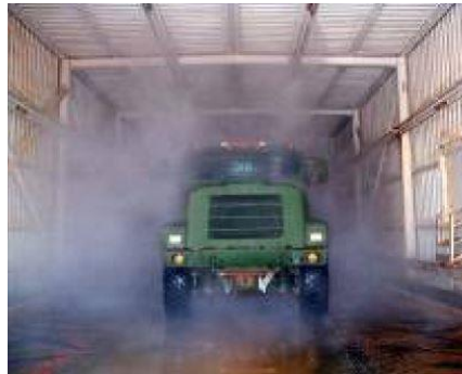
Figure 95. Steam and Water Jet Cleaning (Koch, 2011).
