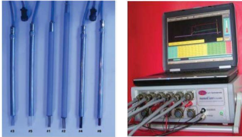
Figure 78. Coupled multielectrode sensors (left), and coupled multielectrode corrosion analyzer (right) (Sun, 2005).
