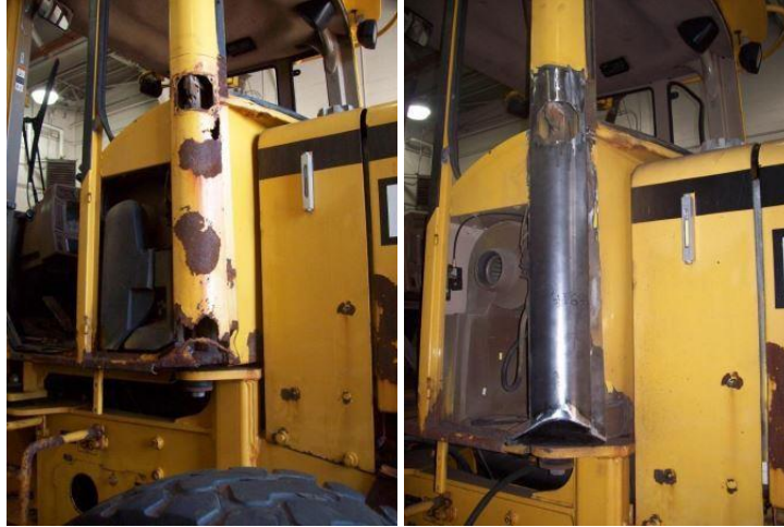
Figure 41. Before rebuild (left), after (right) (Chupas, 2014).
