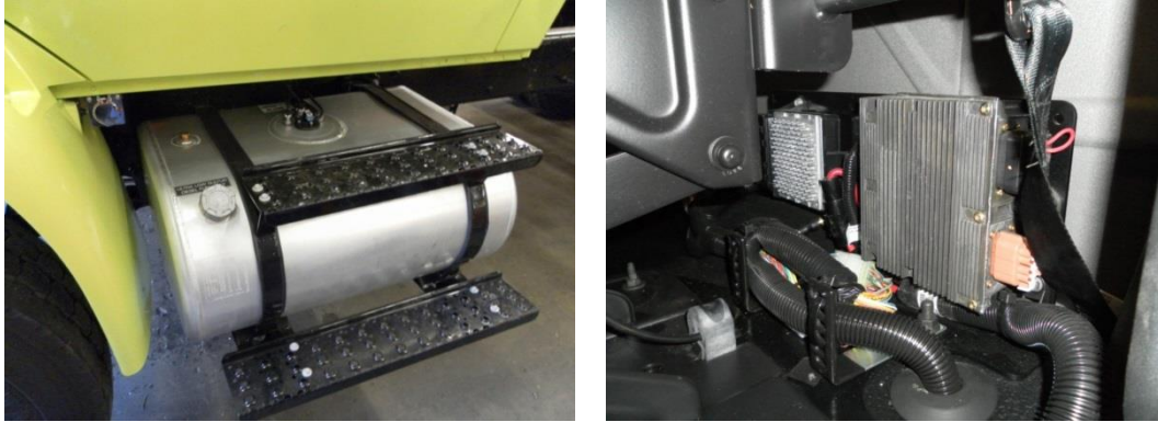
Figure 98. New fuel tank made of aluminum (left), and modified electrical junction boxes which are mounted inside the cab off the floor (right) (Shi et al., 2013).
