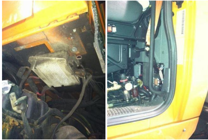
Figure 103. 2007 RPM box mounted under cab (left) and 2010 RPM box mounted behind driver seat (right) (Chupas, 2014).
