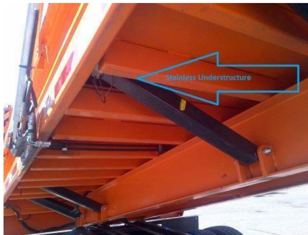
Figure 49. Understructure of stainless steel (Chupas, 2014).
