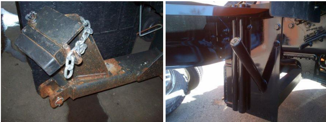
Figure 106. ConnDOT specification requires body builder to completely prime and paint with “Continental” 2 part urethane paint and primer (Chupas, 2014).
