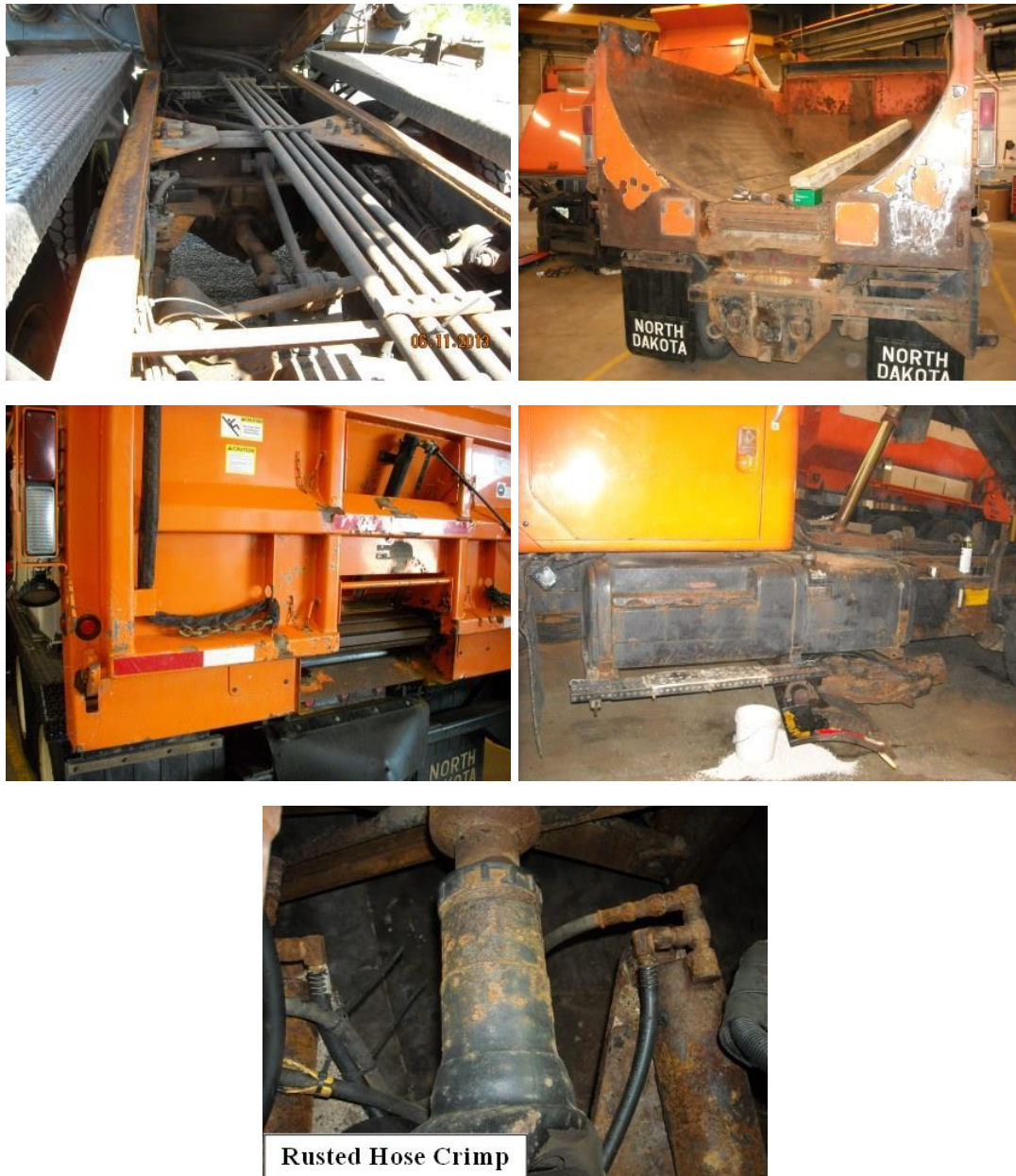
Figure 23. Images of corrosion damages on NDDOT vehicles (courtesy of NDDOT).
