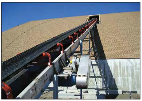
Photo#2: Conveyor systems that fill a salt storage facility from its highest point maximize the facility's capacity and are safer and more efficient than simply pushing salt into a stockpile.
