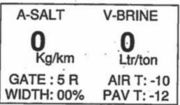
Hold ENTER button down, press ESC button, and let go both buttons at the same time. Press ESC to switch to OPERATOR SCREEN as shown below:
