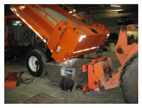
Figure 3. Raising the dump body but make sure the truck or anything else touches the scale
