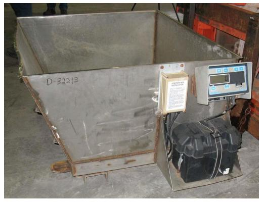
Figure 1. Electronic scale used for calibration
