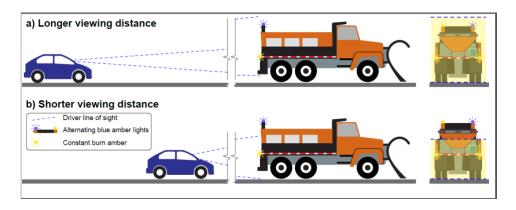
Figure 2.2 Proposed Mounting Location for Steady Burn and Flashing Snowplow Lights
