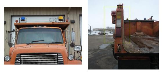
Figure 2.3 Examples of Forward and Rear Snowplow Warning Lights
