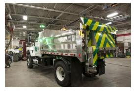
Figure 2.7 Ohio DOT's Combination of Colored Lights for Snowplows
