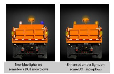
Figure 2.5 New Rear Lighting on Some Iowa DOT Snowplows
