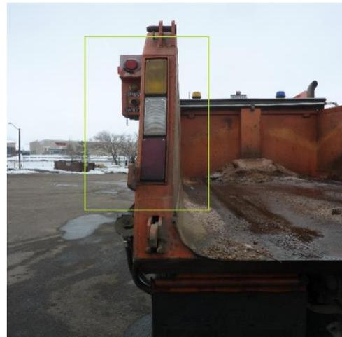
**Figure 2.3 Examples of Forward and Rear Snowplow Warning Lights**
