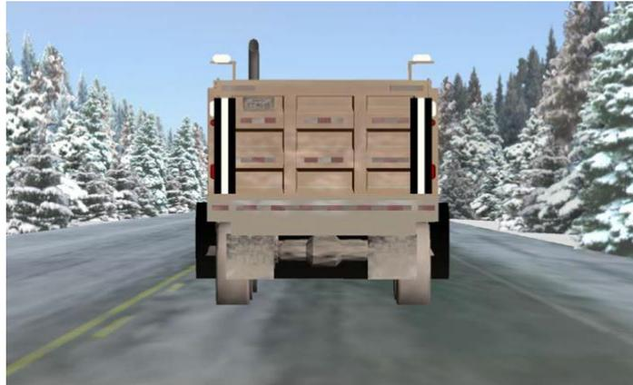
**Figure 2.4 Snowplow Lighting Recommended by University of Minnesota Researchers**
