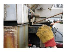
6) The spotter will then remove the spinner and chute assembly locking pin, located at the rear and to the right on the hopper.
