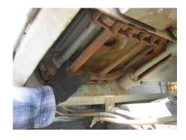
As a final step, check the gear box for proper fluid level.
