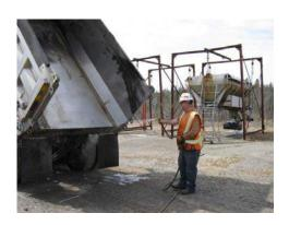
2) During summer use, the body of the truck can become cluttered with gravel, pavement, miscellaneous tools and even an occasional bottle or can. Make certain the body is completely clean of all debris before installing the hopper.
