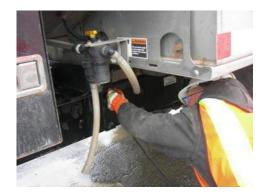
➤ Grease all fittings. These are typically located on each end of the idler sprocket shaft and on the drive shaft, opposite the gear box. Fittings may also be located at the rollers, if so equipped.
