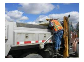
1) When preparing for a winter storm event, check and completely clean the body of all tools, gravel material, pavement, etc.
