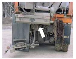
The Precision Placement System (PPS) is manufactured by the Swenson Spreader Company of Lindenwood, Illinois. It is designed to place salt in a windrow pattern at the centerline of the roadway. The PPS is an add-on to our standard hoppers that consists of an auger or chute and a high speed, shrouded spinner
