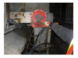
> Check the gear box for proper fluid level.
