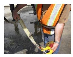
> Connections on the limiter strap must be checked and found to be secure and functional.
