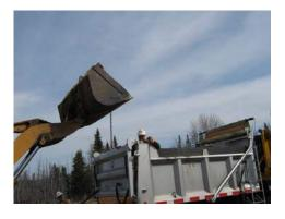
1) The first step in the hopper installation procedure is to remove the tailgate. To achieve this, first move the truck to a designated area to have the tailgate removed using a bucket loader if a tailgate stand is not available. Attach a properly rated lifting chain to the link on the top of the tailgate and apply enough upward pressure to allow the tailgate pins to be removed. After the pins have been removed, check to see that the
