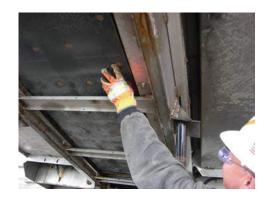
> To complete the maintenance procedure, check the bed chain or belt for proper tightness and alignment.
