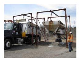
9) The operator will raise the body until there is slack in the front chain that suspends the hopper in the gantry. The spotter will notify the operator that they are climbing between the cab and body to release the front chain. Note: The chain should be hooked to the gantry so as to clear the hopper when driving away.
