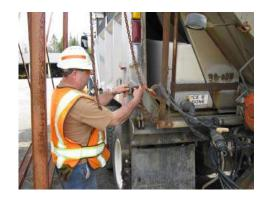
7) The spotter will close and lock the tailgate latch and hook the two safety chains located at either side of the rear of the hopper.
