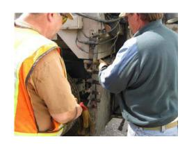
16) Connect all wiring for lighting, controller (Compu-Spread, Cirus, Schmidt), etc. Note: Check the controller connector to assure a liberal amount of dialectic grease is present.
