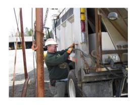
13) Connect all wiring for lighting, controller (Compu-Spread, Cirus, Schmidt), etc. Note: Check the controller connector to assure a liberal amount of dialectic grease is present.
