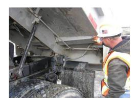
Next, complete a visual inspection of the body. Check all welds, bolts, etc.
