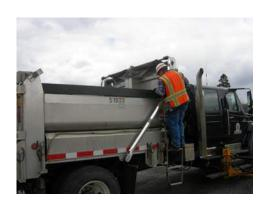
1) When preparing for a winter storm event, check and completely clean the body of all tools, gravel material, pavement, etc.
