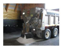
1) To begin the hopper removal procedure, position the vehicle at the appropriate stockpile location and completely empty the hopper of all granular material.
