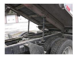
> Lift the dump body and place dump props into position
