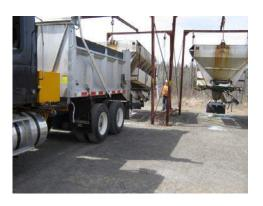
5) With the truck body in the down position and at the direction of the spotter, the operator will slowly back under the hopper so as to allow the hopper to slide into the truck body.
