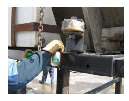
> Front, side and rear rollers should receive a liberal application of chain and cable lube.
