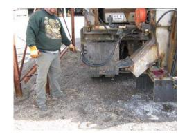
17) Check for hydraulic leaks.
