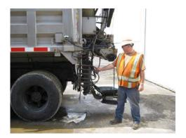
21) To complete the installation process, make one final and overall check of the hopper to confirm safety chains, hydraulic fittings and electrical connections are properly attached.
