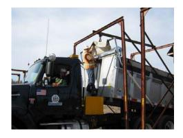
7) The spotter will then notify the operator that he is going to climb between the cab and body of the vehicle to attach the front chain.
