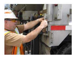
14) Next, the operator and spotter will completely secure the hopper by fastening all the safety chains and latches provided. These should consist of two sets of safety chains; one on either side of the bottom rear corners and a chain and binder located on each of the front upper corners. Note: When tightening the front binders use caution not to over tighten, as this can cause damage to the hopper.
