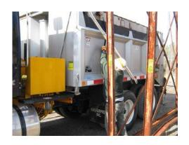
5) At this point, the operator and spotter will remove the safety chains and binders from the front of the hopper and safety chains from the rear of the hopper.
