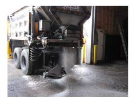
1) To begin the hopper removal procedure, position the vehicle at the appropriate stockpile location and completely empty the hopper of all granular material.
