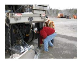
6) The operator and spotter will remove the rear leg locking pins, lower the rear legs into position and reinsert the locking pins.
