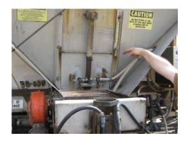
18) Confirm the gate is positioned at the proper gate setting.
