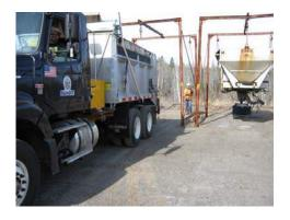
3) Under the direction of the spotter, the operator will slowly back the truck under the desired gantry system. The spotter will take particular care to position the truck directly under the hook points to assure the hopper is lifted straight off the truck body. The spotter will direct the operator to secure the vehicle by putting the truck in neutral and applying the parking brake. Note: It is now safe for the operator to exit the vehicle and assist the spotter.
