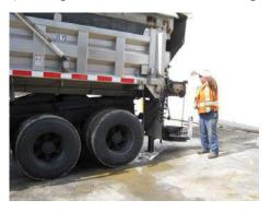
13) With the truck already secured, it is now safe for the operator to exit the vehicle and assist the spotter with unpinning, lifting and re-pinning the rear legs of the hopper stand unit.
