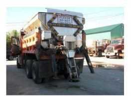
Each of these spreaders is stored using a hopper stand system. The modified spreaders are installed and removed in the same manner as the standard hoppers, while the Stratos system has one additional requirement. The chute/spinner assembly must be raised when removing the spreader. This additional step is documented as step 4A in the <u>Hopper Removal (Hopper Stand System)</u> section.
