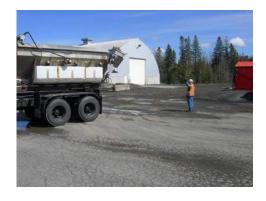
4) Move truck to the desired drop location. Under the direction of the spotter, the operator will slowly back the truck into position. The spotter will direct the operator to secure the vehicle by putting the truck in neutral and applying the parking brake. Note: It is now safe for the operator to exit the vehicle and assist the spotter.
