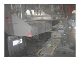
3) The next step is to install the spinner assembly.
