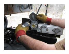
10) Next, the spotter will disconnect the electric winch connector. Note: Before completing this step, make certain the winch cable is tight and lying firmly against the back of the chute assembly.
