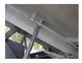
> Lift dump body and place dump props into position
