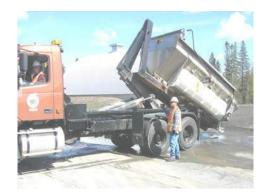
4) With the hopper just off the ground, the spotter will direct the operator to apply the parking brake and complete the loading process.
