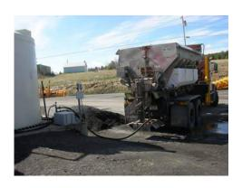
2) Next, position the vehicle at the storage tank area and completely empty the liquid storage tanks. Rubber gloves and face shield must be worn Note: A potential spilling hazard exists if liquid is present in tanks during the hopper off-load. Shifting liquid can spill out from the over-fill tubes during removal.
