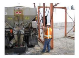
11) The spotter will raise the hopper utilizing the chain falls until the rear of the hopper has lifted slightly off the dump body floor.
