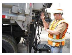
10) At the direction of the spotter, the operator will continue to slowly back the truck while slowly lowering the body until the tailgate latch contacts the pins of the hopper stand and the spotter directs the operator to stop. The operator will secure the vehicle by putting the truck in neutral and applying the parking brake.
