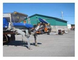
4A) For the Schmidt Stratos Spreader, the chute/spinner assembly must be raised when removing the hopper.
