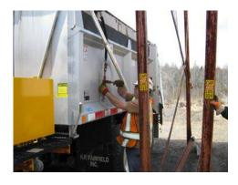
11) With the truck already secured, the operator can safely exit the cab and assist the spotter in hooking the two remaining chains and binders located at the front upper corners of the dump body. Note:
