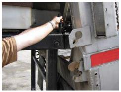
9) The spotter will then direct the operator to back up slowly. The front legs will fold up as the hopper continues to roll into the truck body. Note: Spotter should make certain the limiter strap does not get pinched or cut as the hopper is placed into the truck.
