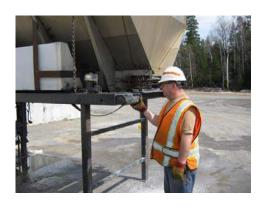
The hopper stand will be inspected for cracks, cracked welds, bent legs and pins, excessive corrosion or other deficiencies that can potentially cause the hopper stand to fail.
