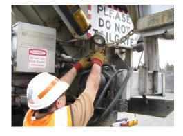
8) With the assembly in the full upright position, the spotter will then hook the safety chain to secure the spinner/chute assembly.
