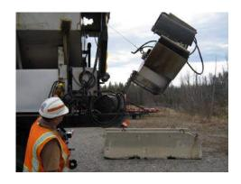
8) The spotter will then operate the winch controls to lower the spinner/chute assembly. Note: At no time will any person stand under the assembly during this procedure.
