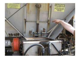
15) Confirm the gate is positioned at the proper gate setting.
