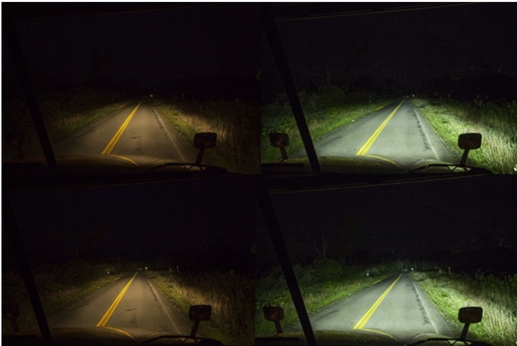
Figure 1: Comparison between Halogen and LEDs lights with high and low beam ( www.truckinginfo.com )
