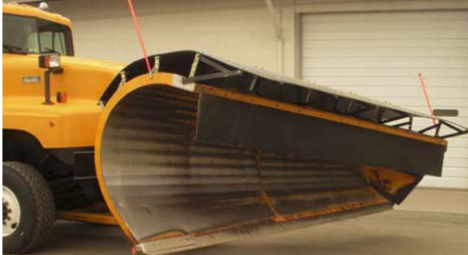
Figure 6: Over plow Deflector (NDOT, 2015)
