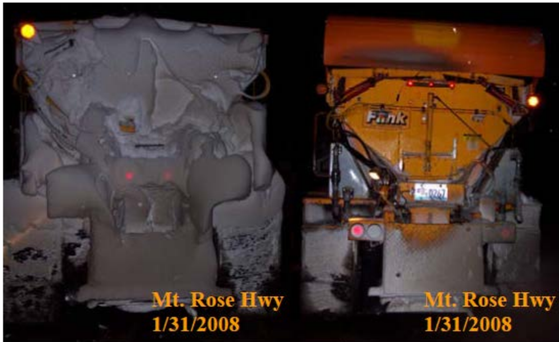
Figure 12: Airfoil test run – without airfoil and more snow accumulation on the rear (left); with airfoil and more snow accumulation on the rear (right) (Nevada DOT, 2015).
