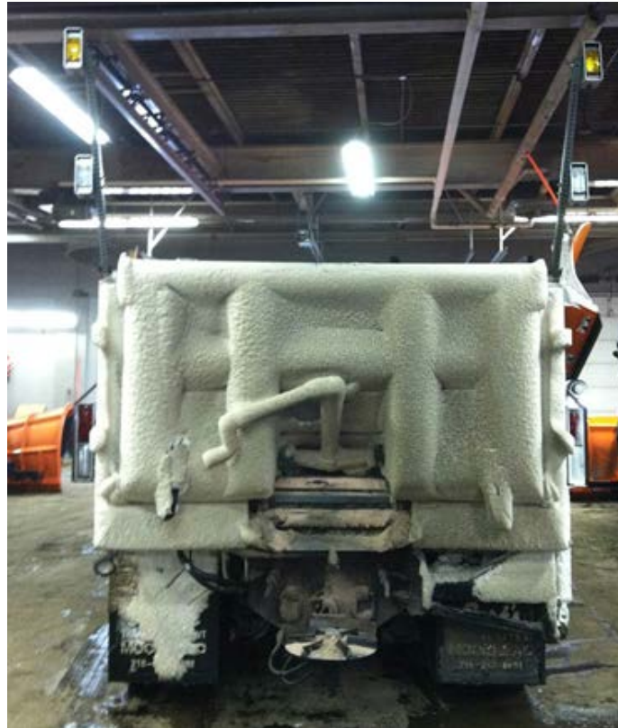
Figure 9: Rear warning lights mounted on the telespar and snow accumulation
