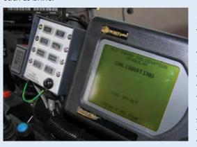
A ground-speed controller in calibration mode.
