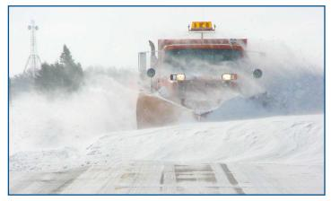
Survey respondents identified several strategies for eliminating snow and ice buildup on truck windshields, including plow deflectors and flaps, heaters and defrosters, heated windshields, chemical glass treatments, and winter-grade wipers.
