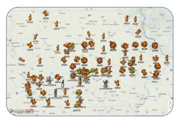
Iowa DOT's SkyHawk tracking software uses AVL/GPS technologies for year-round applications, such as identifying the location of maintenance vehicles, performing equipment checks, and collecting materials and engine data.
