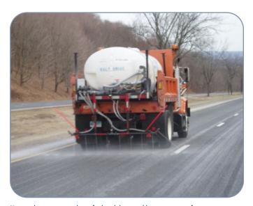
New application rate guidance for liquid deicers addresses a range of pavement temperatures, temperature trends, road surface conditions and materials used.
