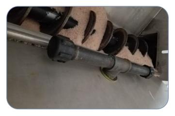
A screw conveyor mounted inside a truck pre-wets dry salt before it's applied to the road. (Photo courtesy of North Dakota DOT.)
