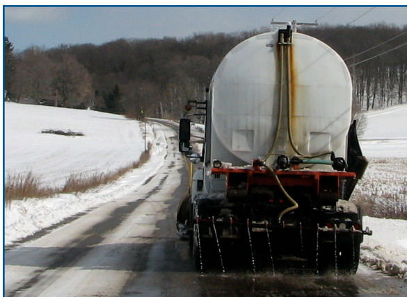
During-storm direct liquid application can be an effective addition to an agency's winter maintenance toolbox, especially for use in milder weather.
