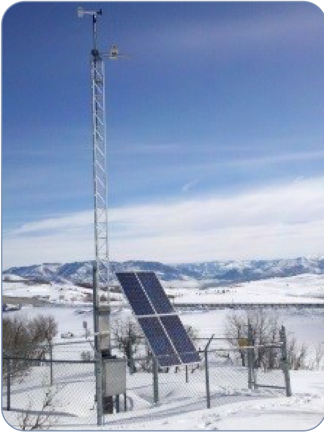
Roadside environmental sensor stations collect data on air temperature, wind speed and direction, precipitation, visibility, and other variables used in severity indexes. (Photo courtesy of Utah DOT.)
