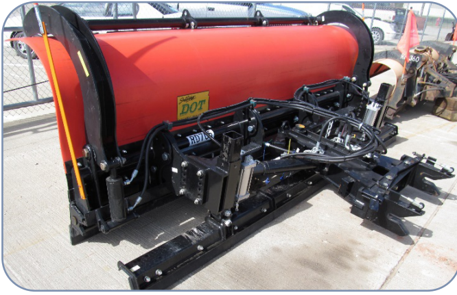
A plow blade with a squeegee blade mounted behind the carbide cutting edge is among many alternative winter maintenance technologies and techniques for transportation agencies to consider. (Photo courtesy of South Dakota DOT)
