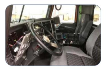
A typical snowplow cab features an array of controls and electronic instrumentation. The Clear Roads Plug-and-Play Initiative improves the interoperability of this equipment across manufacturers and agencies.
