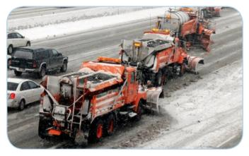
Common equipment for winter road maintenance includes snowplows with hopper-type spreaders (lower left) and trucks that hold tanks of liquid deicers (upper right). Photo courtesy of Utah DOT.
