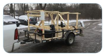
Researchers built an adjustable rig onto a trailer to allow all four mobile sensors to be tested simultaneously, each at its optimum mounting height. The rig was used in live traffic as well as closed-course testing.
