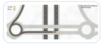
This is an image from the manual and training video: an animated sequence shows the plow path for clearing a Double Roundabout Interchange. The icon in the upper left-hand corner shows that this is the path of Truck #1 on Pass #3 of the clearing sequence.
