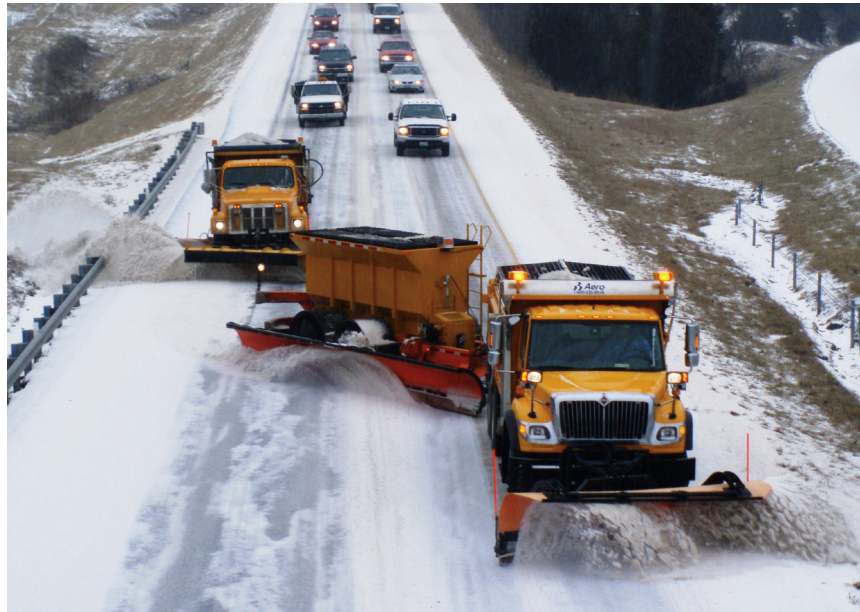
Some transportation agencies use innovations such as the tow plow, which can clear two lanes of a road simultaneously, to improve snow removal operations.
