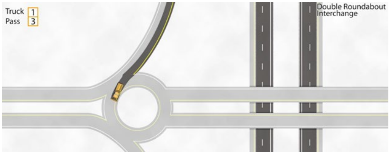
Figure 6.2: snow plowing pattern for the Pass 1/3 (a)
