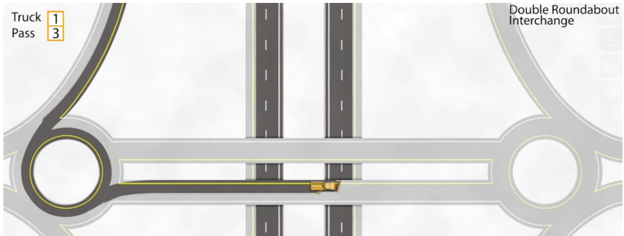
Figure 6.4: Snow plowing pattern for the Pass 1/3 (c)
