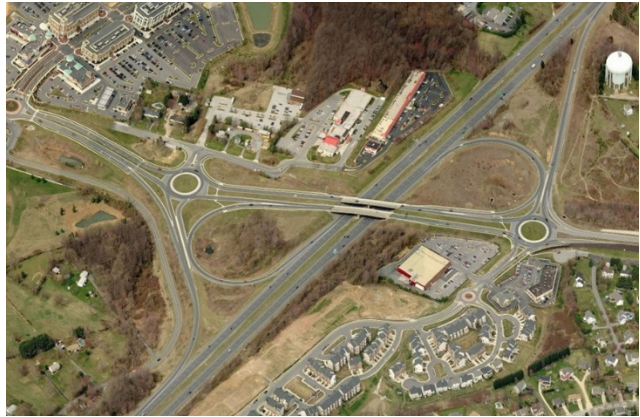
Figure 6.1: Double roundabout interchange
