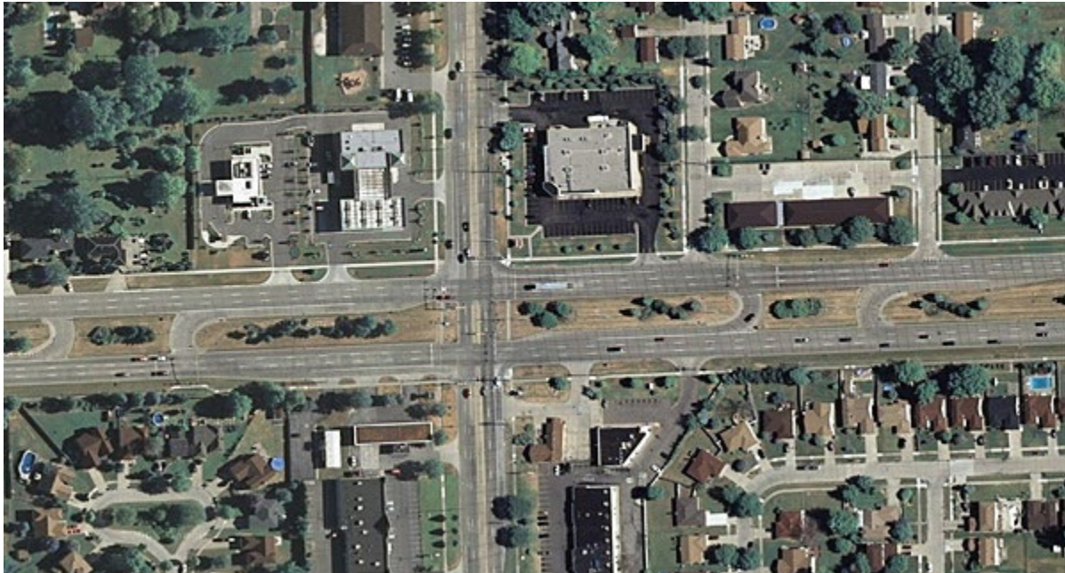
Figure 5.1: Median U-turn intersection
