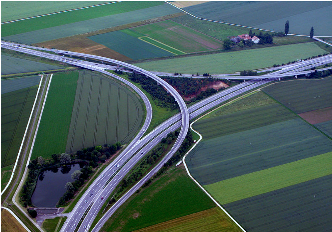
Figure 11.1: Directional T interchange
