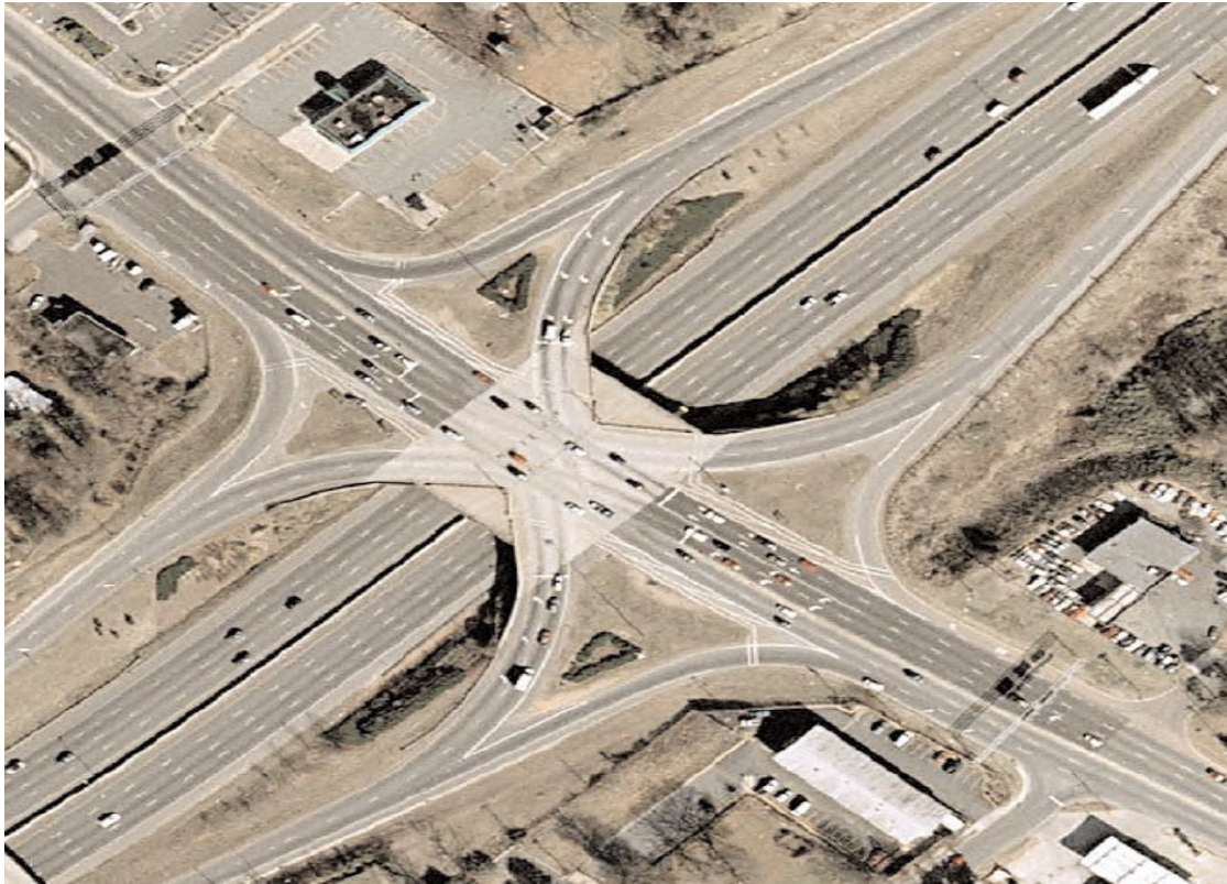
Figure 9.1: Single point interchange
