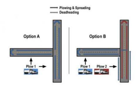
The results of snowplow route optimization can vary depending on an agency's service priorities. The option on the left uses a single plow to achieve lower costs. On the right, the same route can be cleared more quickly with two plows working together. Image courtesy of Clear Roads.
