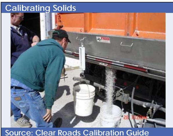
Also check during operations that spinner or chute is not plugged, that material is coming out of the spinner at the expected rate. More extensive pre-season inspections are vital to ensure vehicles and equipment will be ready well in advance of winter. Post-storm and post-
