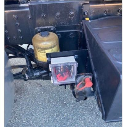
Figure 12. Junction Box at Battery Box
