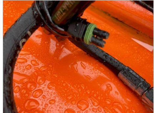
**Figure 9. Installed Weather Pack Connector**
