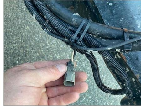
**Figure 4. Portion of Deutsch Connector Assembly on Wing Plow**
