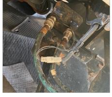
Figure 5. Deutsch Connector on Wing Plow (Source: Delaware DOT)
