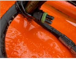
**Figure 9. Installed Weather Pack Connector** (*Source*: Vermont Agency of Transportation)
