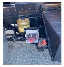
Figure 12. Junction Box at Battery Box (Source: Delaware DOT)
