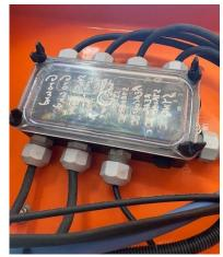
Figure 13. Junction Box in Tow Plow (Source: Delaware DOT)
