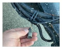
Figure 4. Portion of Deutsch Connector Assembly on Wing Plow (Source: Delaware DOT)
