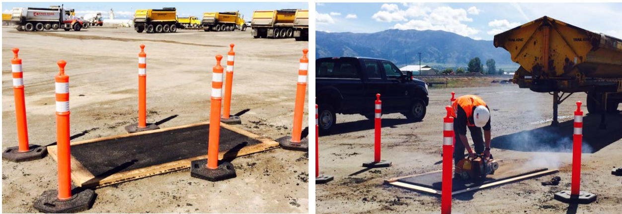
Figure 5: DGP compacted in wood form (left) and cutting samples (right).
