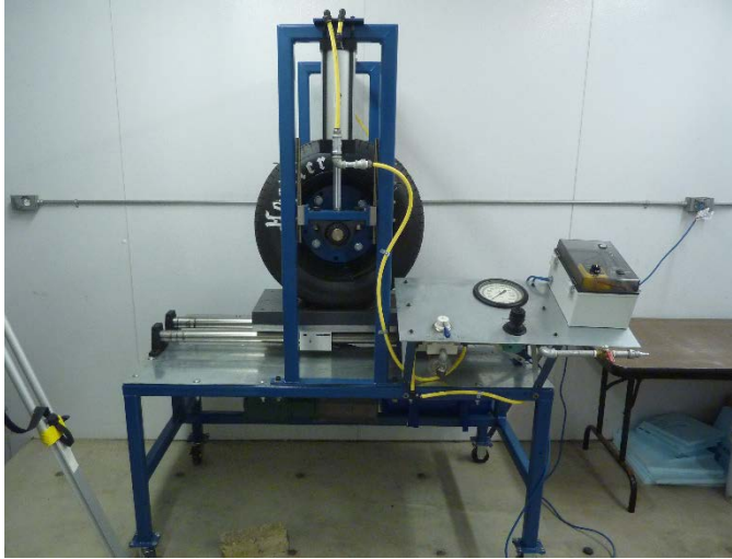
Figure 15: Simulated trafficking device.
