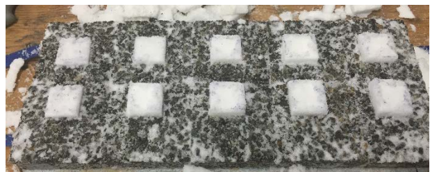
OGFCma5y Dry Salt test
