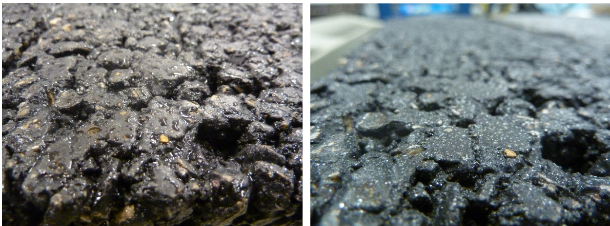
Figure 13: Close-up of a pavement sample after applying salt brine (left) and after drying (right).
