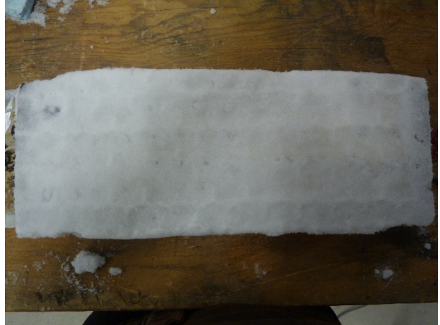
Figure 16: UTFC-ny sample during a deicing test with dry salt before and after trafficking.
