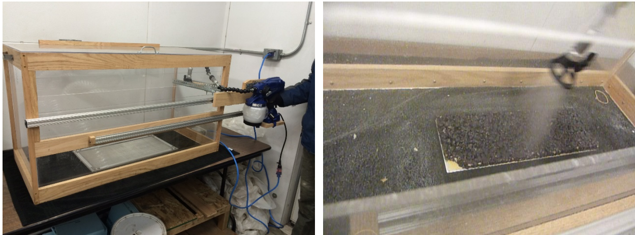
Figure 12: Enclosure and sprayer for anti-icing pavements.
