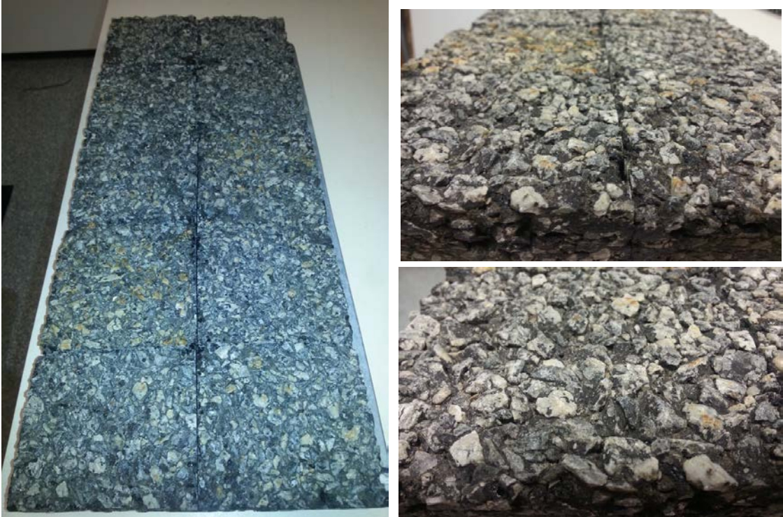
Figure 9: Open-graded friction course pavement from Massachusetts cores (OGFC-ma5y).
