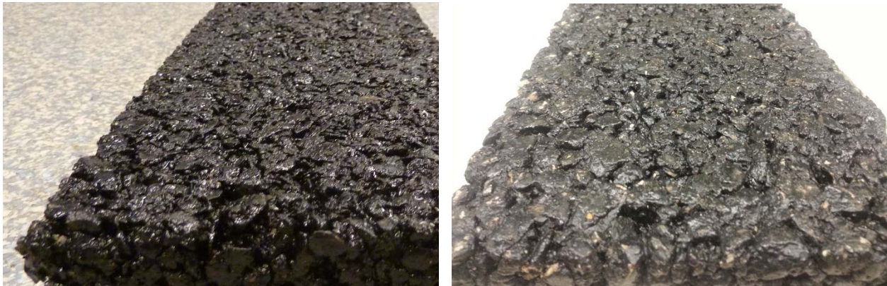
Figure 7: Ultrathin friction course pavements made with pavement mix from New York with \frac{1}{2} inch max aggregate (left) and Missouri with \frac{3}{4} inch max aggregate (right).
