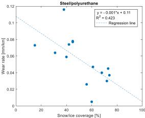
Figure 4-15: Correlation of Wear Rate and Snow/Ice Coverage for Nordic Combi Double Blades
