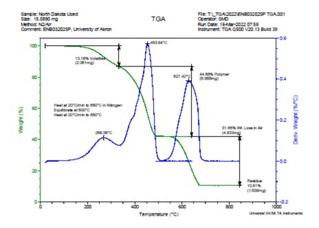
Figure 4-36: TGA Thermogram Obtained on the North Dakota -- Used Polymer Component
