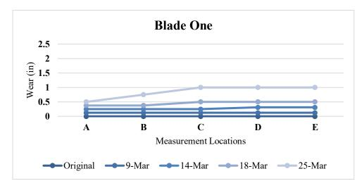
Figure 4-4: Blade One tested in Soda Springs
