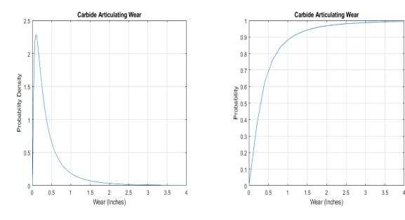
Figure 5-12: Carbide Articulating Wear Probability Density Distribution
