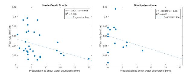
Figure D-0-12: Scatterplot of the wear rate versus the amount of fallen snow (in mm water equivalent)
