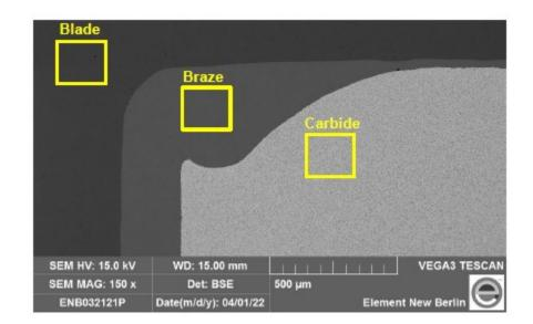
A BSE scanning electron micrograph of the Iowa cross-section is presented in Figure 4-21.
