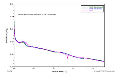
Figure 4-34: Overlay of the DSC Thermograms Obtained on the Three Polymer Components During the Second Heating Cycle
