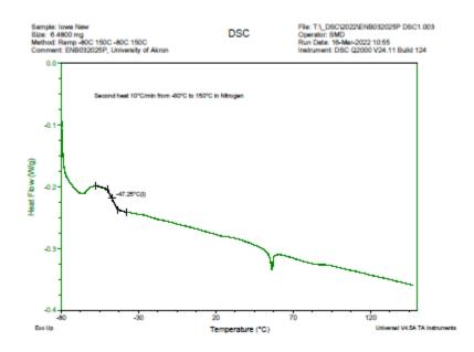
Figure 4-33: DSC Thermogram Obtained on the Iowa Polymer Component During the Second Heating Cycle
