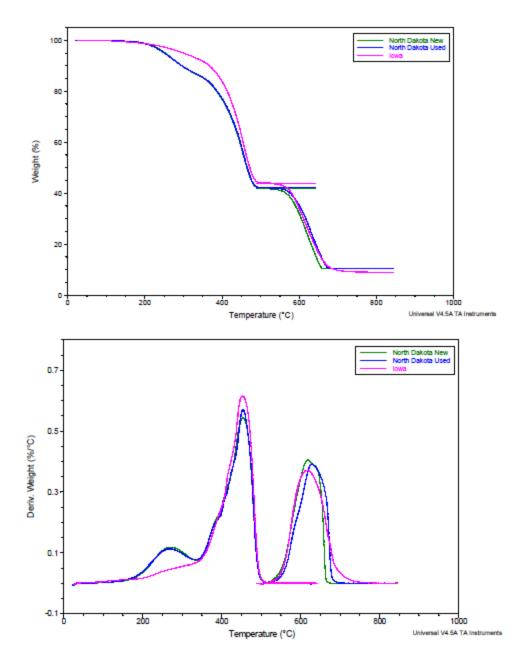
Figure 4-38: Overlay of the TGA Thermograms
