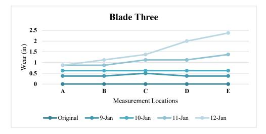
Figure 4-7: Blade Three tested in Soda Springs
