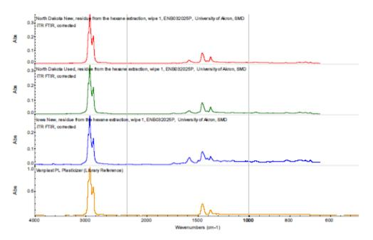
Figure 4-30: FTIR Spectra Obtained on the Hexane Residues of the Blade Polymer Components
