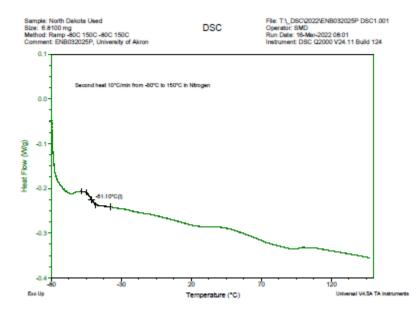
Figure 4-32: DSC thermogram Obtained on the North Dakota – Used Polymer Component During the Second Heating Cycle
