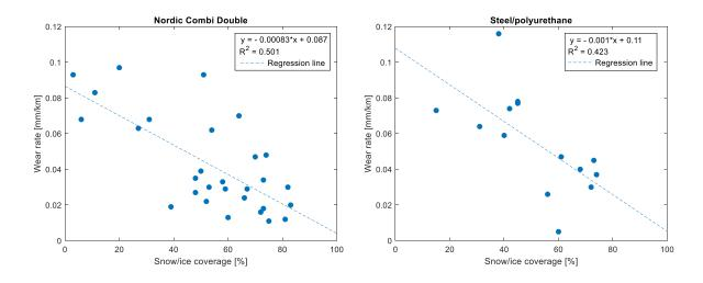
Figure D-0-16: Scatterplot of the wear rate versus the snow/ice coverage
