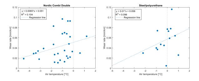
Figure D-0-14: Scatterplot of the wear rate versus the air temperature
