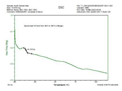
Figure 4-31: DSC thermogram Obtained on the North Dakota – New Polymer Component During the Second Heating Cycle
