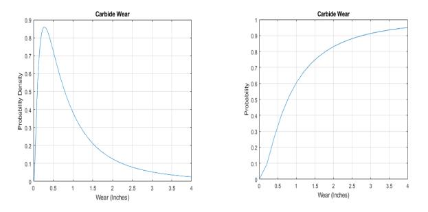
Figure 5-8: Carbide Wear Probability Density Distribution Figure 5-9: Carbide Wear Cumulative Distribution
