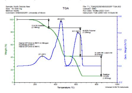
Figure 4-35: TGA Thermogram Obtained on the North Dakota – New Polymer Component
