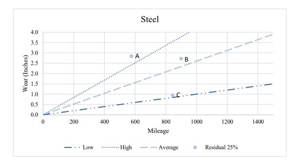
Figure 5-5: Steel Blade
