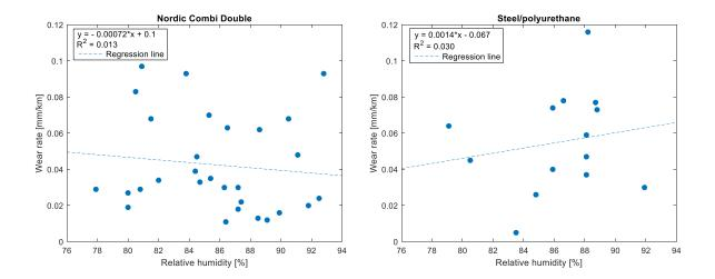
Figure D-0-15: Scatterplot of the wear rate versus the relative humidity
