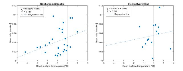
Figure D-0-13: Scatterplot of the wear rate versus the road surface temperature
