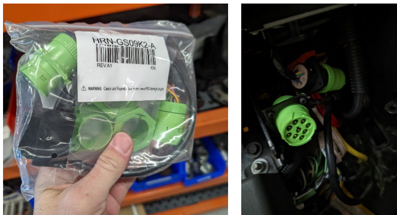
Figure 6. Geotab Vehicle T-Harness with 9-Pin Connector for Heavy Duty Vehicles
