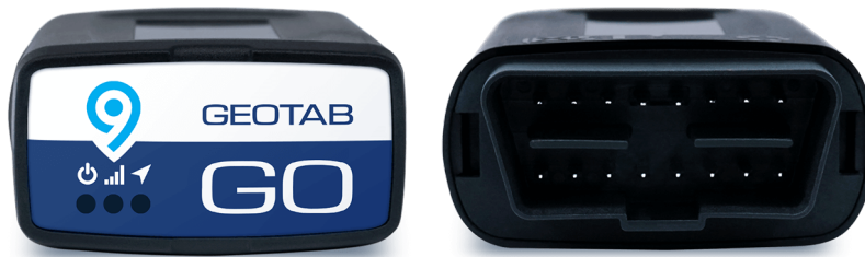
Figure 2. Geotab GO9 Vehicle Hardware (Front and Back) for Vehicles with OBD-II Port
