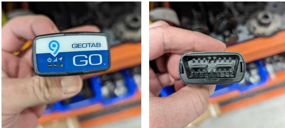
Figure 5. Geotab GO9 Vehicle Hardware (Front and Back) for Vehicles with OBD-II Port
