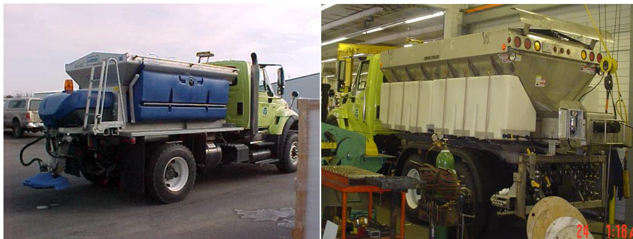
Figure 3-5: Schmidt (left) and Monroe (right) prewetting spreaders (Washington State Department of Transportation photos)
