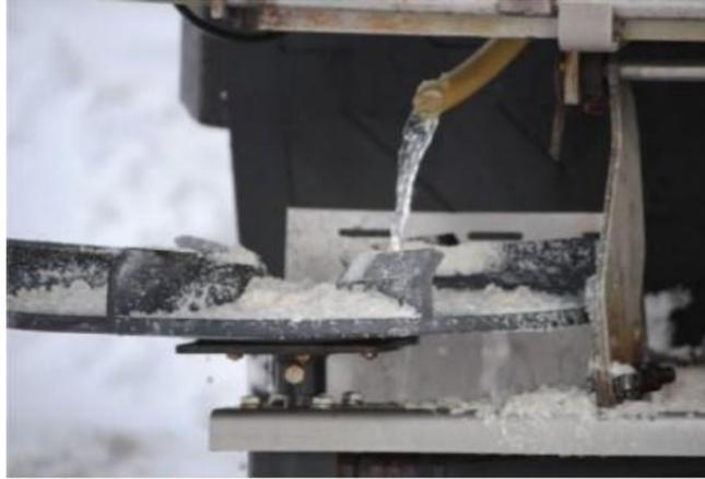
Figure 2.6. Basic on-board pre-wetting operation (Minnesota DOT)
