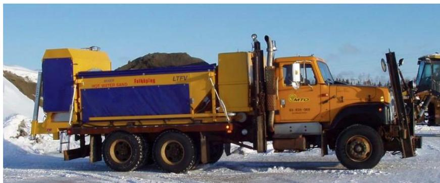
Figure 2.5. Hot water sander (Perchanok et al., 2010)
