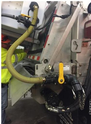
Figure 3.4. The yellow hose with a diameter of 1"
