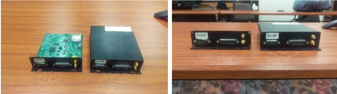
Figure 13. WSDOT AVL/GPS System Hardware Units (Un-covered and Covered)
