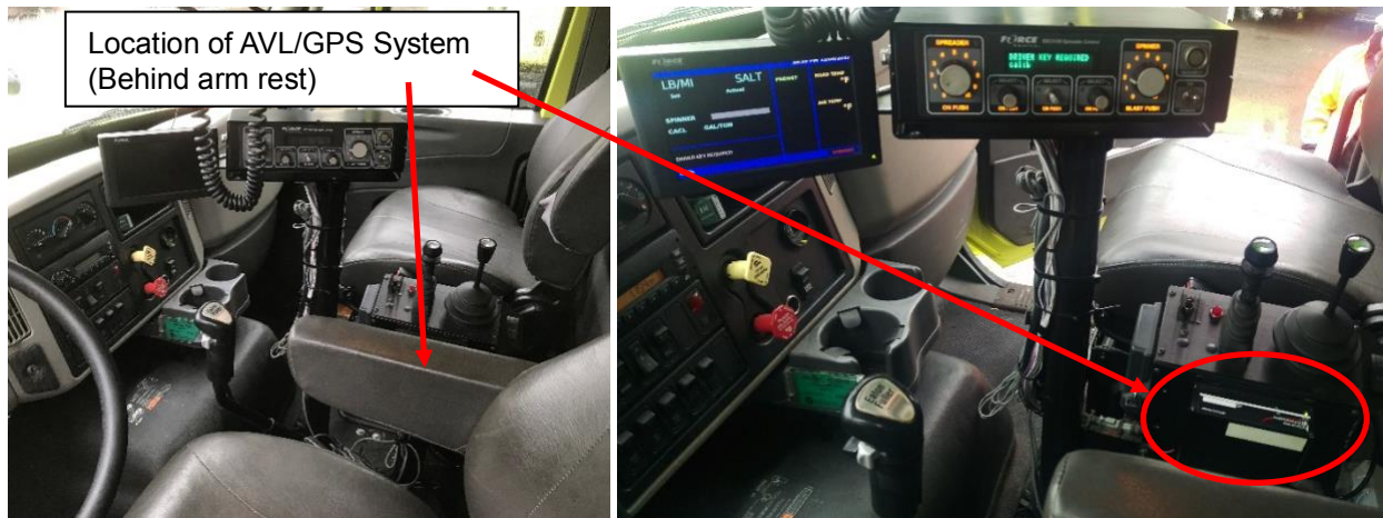
Figure 14. WSDOT Snow Plow Equipment and Location of LT6 AVL/GPS System
