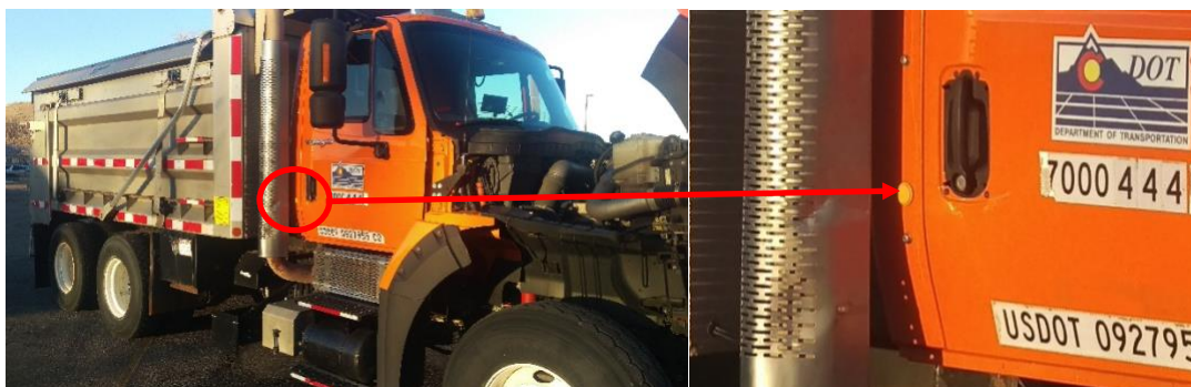
Figure 37. CDOT Snow Plow and Example Reporting Puck for Pre-Trip and Post-Trip Reports
