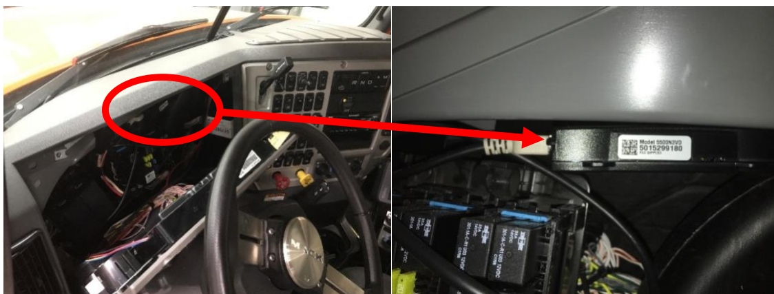
Figure 5. Location of Verizon NetworkFleet 5500 Model in UDOT Snow Plow
