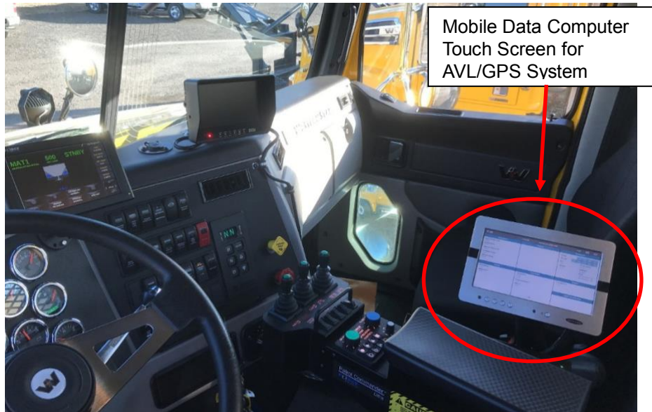
Figure 31. NDOT Snow Plow In-Vehicle Equipment
