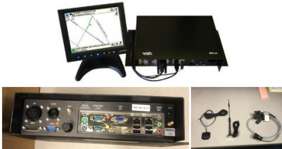
Figure 18. MDOT Mobile Data Computer (MDC) and AVL Hardware (above) and Back View of MDC, Antennae and Cable (below)
