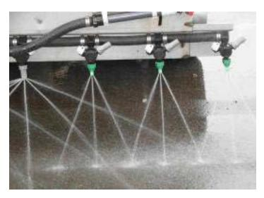
Figure 6: Application of anti-icing solution by nozzles (MDOT Strom Water Management Team & Tetra Tech 2006)
