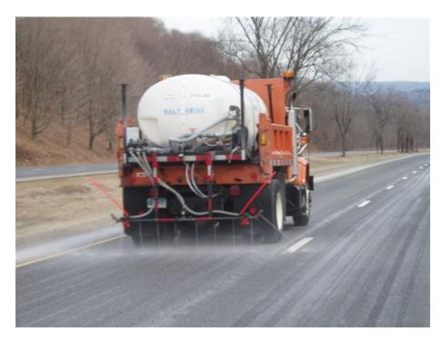
Figure 4: A typical anti-icing operation on dry pavement (Connecticut DOT)
