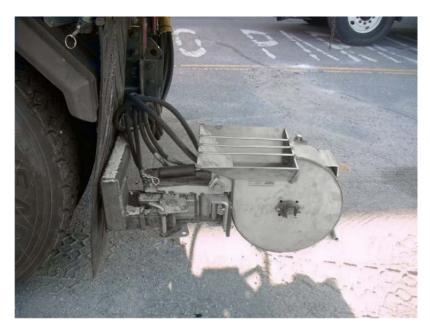
Figure 9: Zero-velocity spreader equipped on a truck (Thompson Engineering Company 2014)
