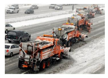
Figure 5: Snowplows with hopper-type spreaders (right lanes) and "all-liquid" truck (center lane). Photo courtesy of Utah DOT
