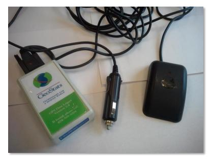
Figure 7 GeoStats GeoLogger (I. to r.) datalogger, 12V adapter, and antenna
