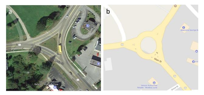
Figure 8 The intersection of US 2 and US 3 in Lancaster, New Hampshire as a stop- and yield-controlled intersection (a) and as a roundabout (b)
