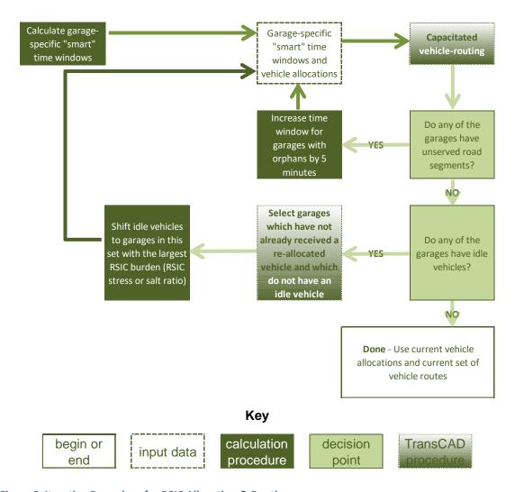
Figure 3 Iterative Procedure for RSIC Allocation & Routing
