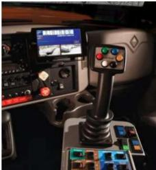
Figure 3 – Cirus's Joystick with a SpreadSmart Rx Color Display (Source: Cirus 2014)
