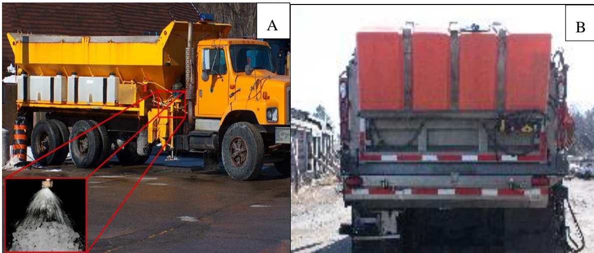
Figure 45: On board pre-wetting apparatus A) side mounted and B) tailgate mounted tanks (Photo credit: www.MeltSnow.com and Wilkinson Corp.)
