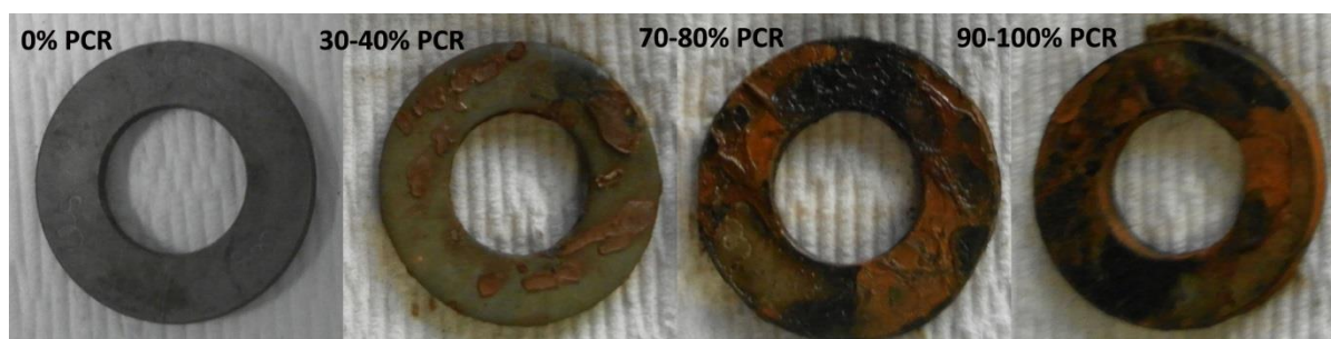
Figure 29: Steel coupons after the gravimetric corrosion test showing percent corrosion rate (PCR).
