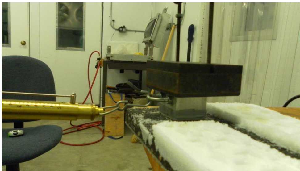
Figure 21: Friction tester measuring the friction after the plow
