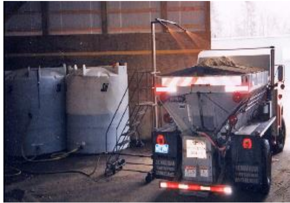
Figure 44: Pre-wetting a load on an out-bound truck. (Photo credit: Wilkinson Corp.)
