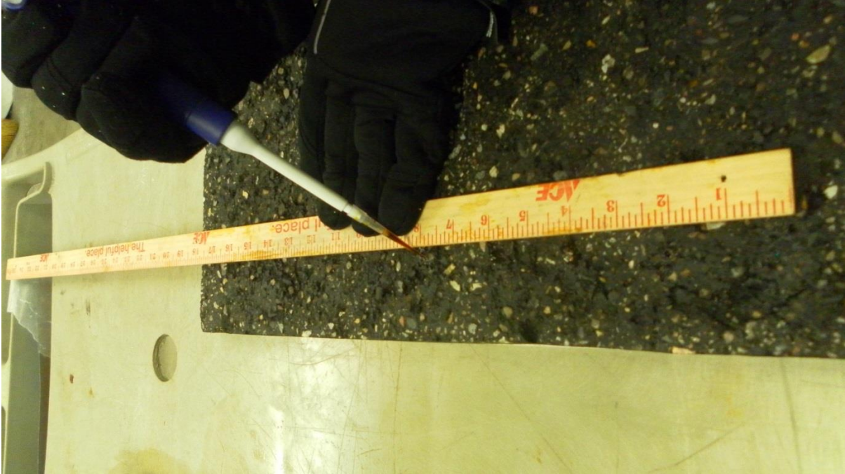
Figure 17: Application of liquid product on pavement sample using a pipette
