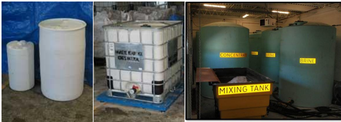
Figure 42: Liquid snow and ice control product storage options: a) drums, b) totes, c) poly tanks
