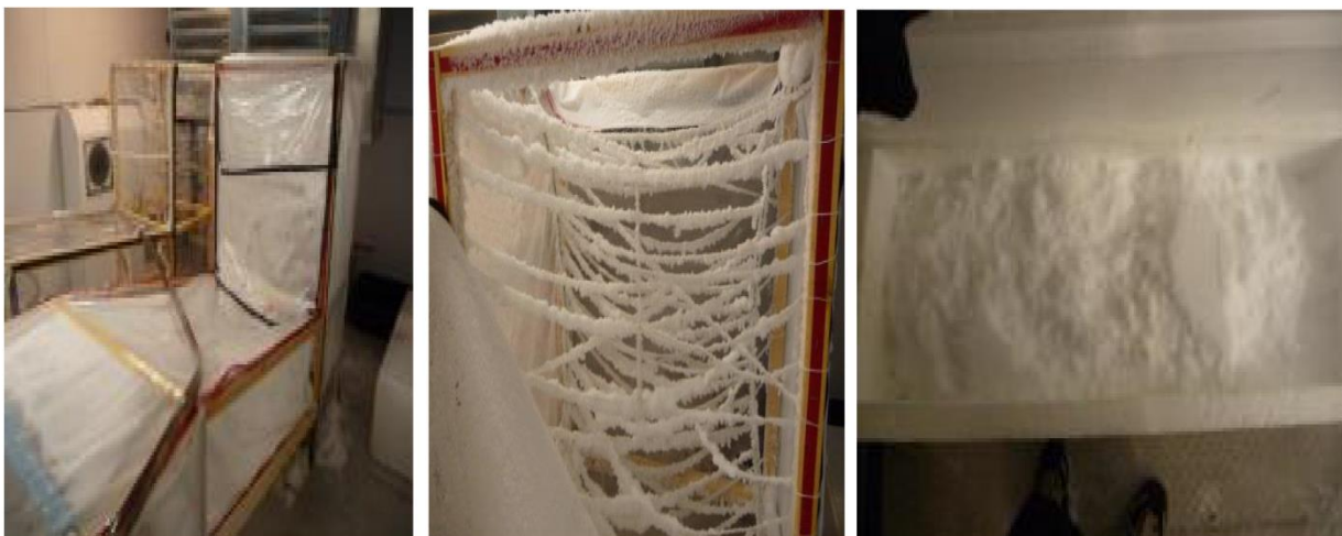
Figure 15: Snow making process and snow storage at the subzero lab
