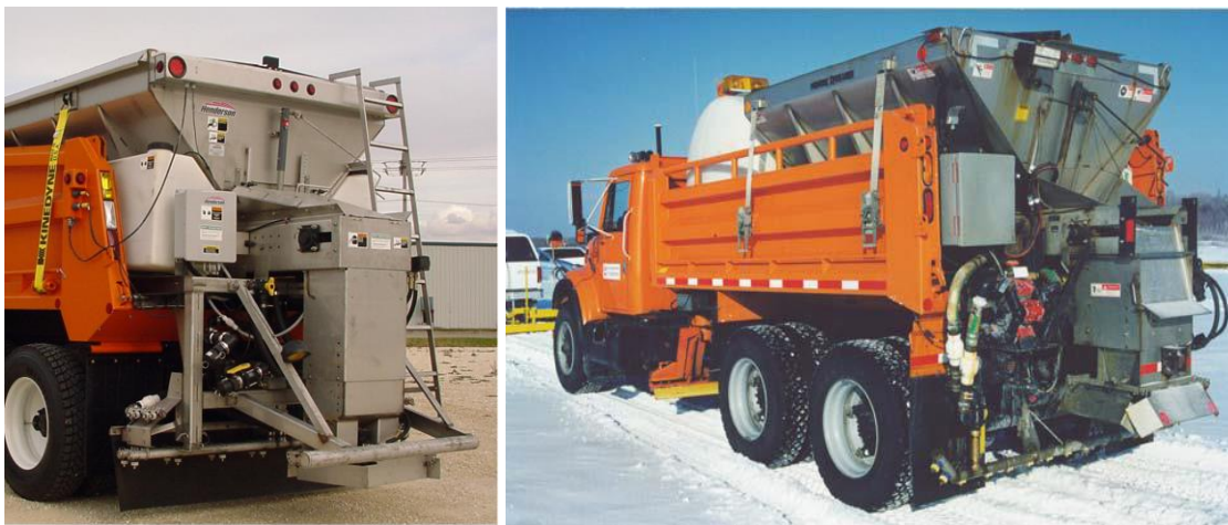
Figure 46: Rear-mounted slurry equipment
