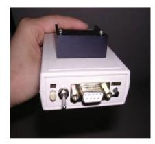
Figure 50. Port and On/Off Toggle Switch on Back of Interface
