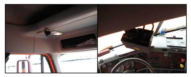
Figure 7. Example of the Dome Camera Mounted on Roof of Cab (left) and View from Behind the Dome Camera (right) providing an Over-the-shoulder View of the Driver, Steering wheel, and Dashboard
