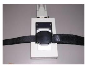
Figure 52. Proper Actigraph Watch Interface Placement for Downloading Data
