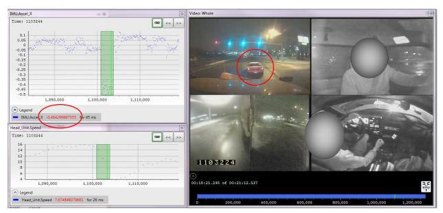
Figure 13. Example of a Validated Trigger where the Longitudinal Acceleration was of Greater Magnitude than the Pre-set Value of |0.20 g|
