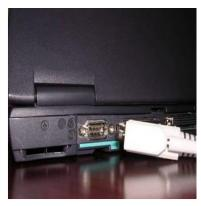
Figure 49. Serial Port on Computer Back
