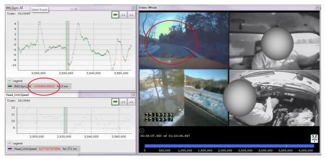
Figure 14. Example of a Non-conflict Event (with a Valid Trigger) where the Driver's Swerve (Quick Steering) was -4.065 (trigger was set to I2.0 gl)
