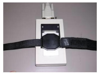
Figure 10. Downloading Data from Actigraph Device
