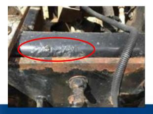
Intergranular corrosion occurs at grain boundaries. (Specifically for stainless steel this occurs in heat affected zones a short distance from the weld.)
