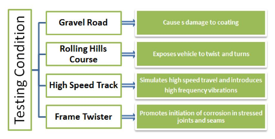
Based on GM tests that accurately simulate 10 years of cosmetic corrosion and 3 years of crevice corrosion
