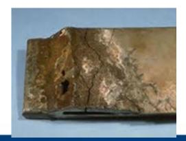
**Corrosion fatigue** is a special kind of SCC caused by the combined effects of cyclic stress and corrosion.
