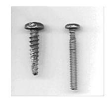
Filform corrosion is a special form of crevice corrosion which happens beneath some types of coatings.
