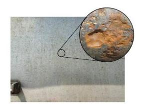
Crevice corrosion occurs at the interface of a metal and another surface, often where a small volume of stagnant solution is contained.
