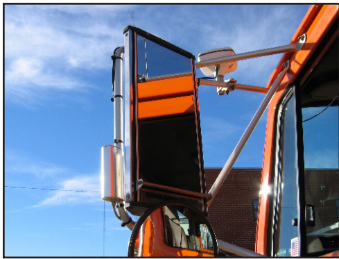
Integrated wiper/washer fluid system for mirrors (photo supplied by Iowa DOT).
