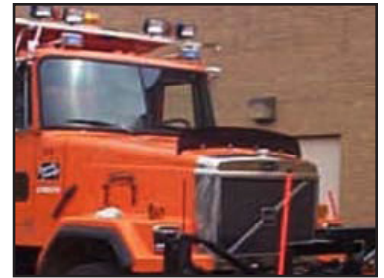
Hood-mounted wind deflector (photo from Wisconsin DOT concept vehicle report).
