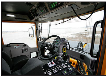
Oshkosh H-Series snowplow with heated windshield—note defroster lines on top and right side of windshield. (photo from Oshkosh brochure)
