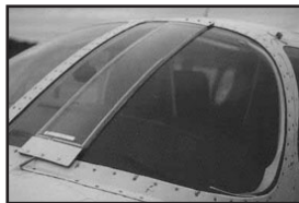
Heated windshield strips for Cessna planes from Maine Aviation Sales (photo from company Web site).
