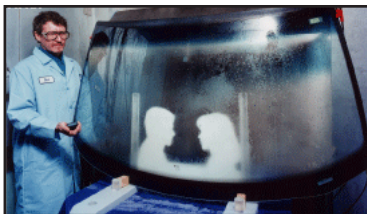
Sungate WeatherMaster heated windshield from PPG (photo from PPG Web site).
