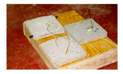
Figure 3-15(a) 1 ft x 1ft x 2 in. slabs
