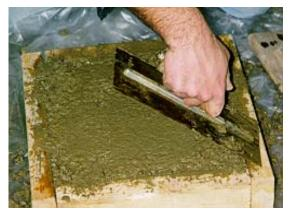
Figure 3-5 Surface finishability of conductive concrete
