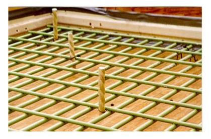
avoid short circuit of electricity during the deicing experiments.
