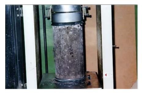
Figure 4-4 Typical failure mode of concrete in compression
