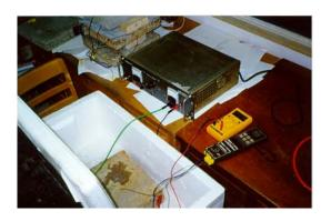
Figure 3-10 Slab under testing using DC-power
