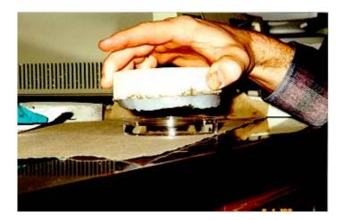
Figure 4-18 Permeability test specimen preparation
