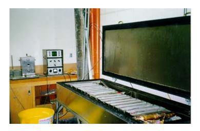
Figure 4-10 Freeze and thaw testing equipment
