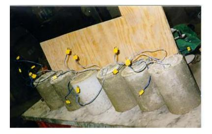
Figure 4-21(a) Cylinders with sawdust mortar insulation layer
