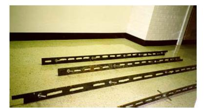
Figure 5-4 Steel plates with opening were used as electrodes The two slabs' dimensions were selected to provide the same volume of conductive concrete overlay for comparison of power requirements.
