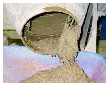
Figure 3-4 Typical conductive concrete mix
