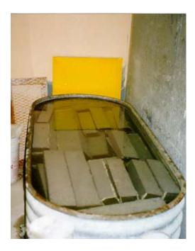
Figure 4-1 Specimens in curing tank
