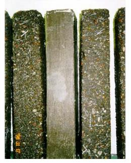
Figure 4-12 Freeze and thaw specimens - before and after 312 cycles
