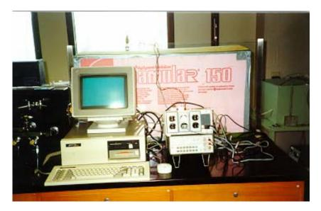
Figure 4-17 Temperature-controlled box for permeability test
