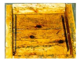
Figure 3-6 Steel plates are used for electrodes
