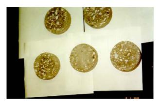
Figure 4-16 One-inch thick specimens for permeability test
