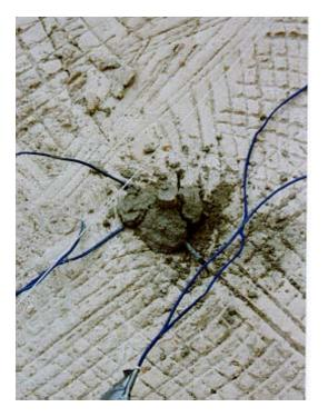
Figure 5-9(a) Thermocouples placed at two levels
