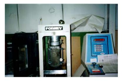
Figure 4-5 Test setup for stress-strain relationship
