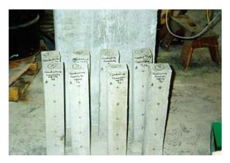
Figure 4-13 Specimens for shrinkage test
