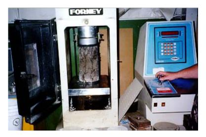
Figure 4-2 400-kip compression testing machine
