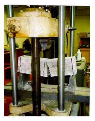
Figure 4-8 Flexural strength - test setup
