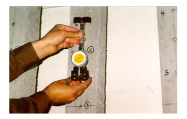
Figure 4-14 Shrinkage strain measurements
