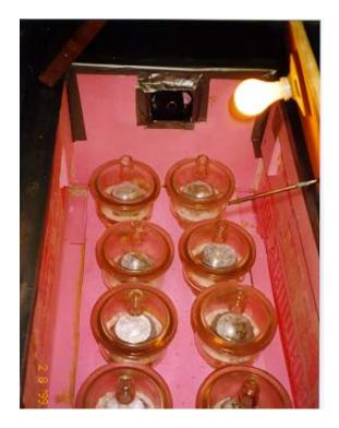
Figure 4-19 Specimens inside moisture-free desiccators
