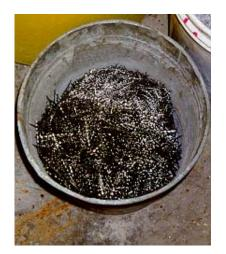
Figure 3-3 Low carbon steel fibers
