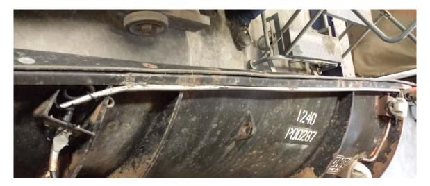
Above: Add on wire protection tube. On the left is the plug and socket connector and it becomes loose after just one 12 hour shift. The plug and socket connections at both ends are replaced on average once every month. The receiving end seems to last longer. These are metal connections.
