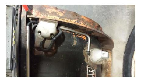
Whelen Lights mounted to a Shop fabricated bracket. These lights also become loose over time. Maybe just a matter of vehicle inspection. Then you cross the line of when is an operator allowed to work as a mechanic. If tightening these lights down is a mechanic's job then the truck is in the shop for repair and not on the road. Should this minor repair be completed by the operator, the truck is still down for a period of time and not in service.
