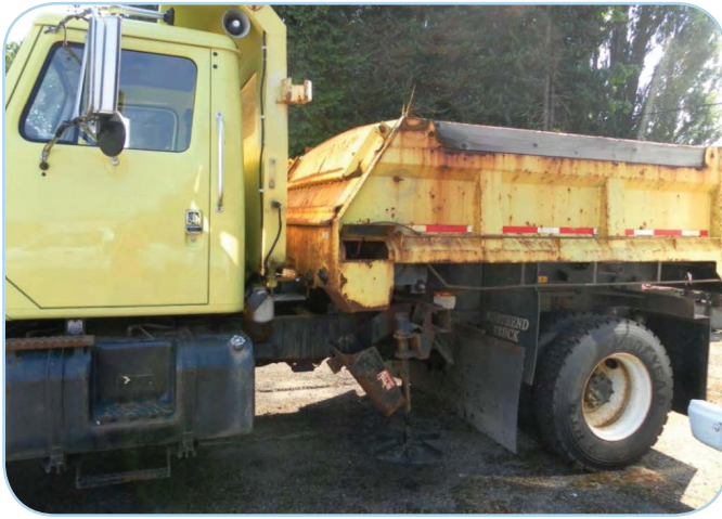
Corrosion of winter maintenance equipment due to deicing agents can increase agency costs by reducing equipment service life, adding repair costs, and increasing equipment downtime.
