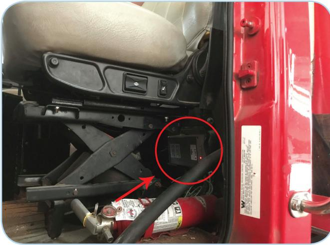
AVL/GPS hardware in this Sawyer County, Wisconsin, snowplow mounts below and behind the seat—a secure position that does not inconvenience the operator.
