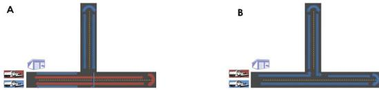
Most survey respondents rated minimizing time until roads are cleared and reducing total vehicle hours as important route optimization goals, although these sometimes conflict. The route on the left, for example, reduces time until clearance by using two plow trucks, but increases total vehicle hours compared to a route serviced by only one vehicle (right).
