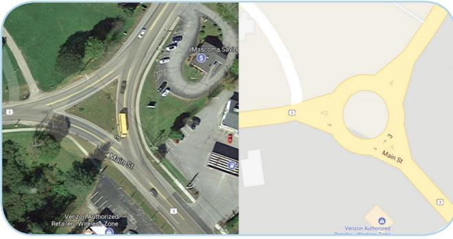
The intersection of US-2 and US-3 in Lancaster, N.H., as (a) a stop- and yield-controlled intersection and (b) a roundabout. The RSIC needs are different for each.
