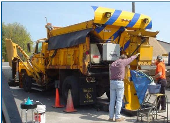
To validate recommended calibration practices, this research took advantage of warm-weather months to carefully capture and measure actual salt output in a controlled setting.
