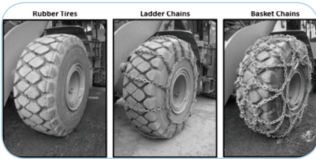
Researchers identified tire chain vibrations as a source of operator fatigue. Basket chains were found to vibrate less than traditional ladder chains.
