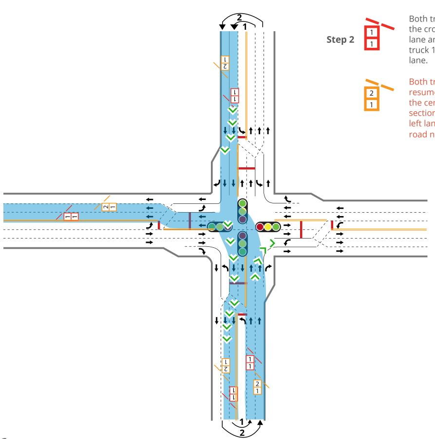
Both trucks turn around and continue **Passes 1/1** and **2/1** on the crossroad, keeping in the formation. Truck 1 in the center lane and truck 2 in the right lane. Crossing the intersection, truck 1 shifts to the left lane and truck 2 shifts to the center lane
