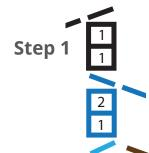
Trucks 1 and 2 begin at near end-point of the main four-lane divided highway. Truck 1; **Pass 1/1** in the left (inside) lane with front-plow angled left and the left-wing plow extended.
