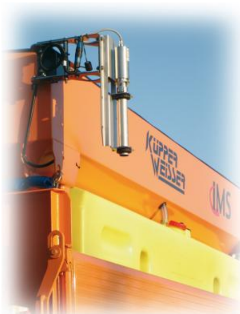
Figure 32: Küpper-Weisser's infrared temperature sensor
