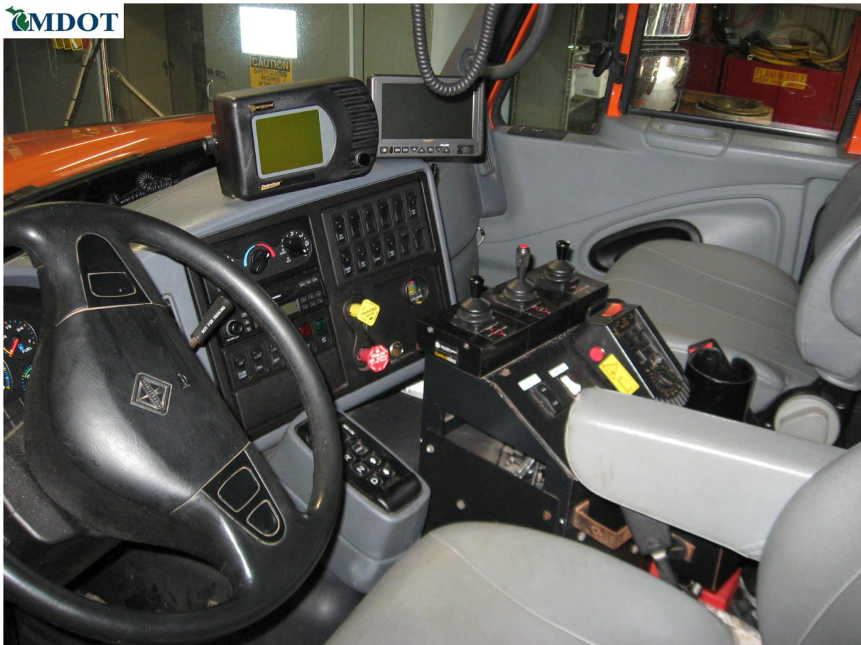
Figure 23: A typical controller setup used by Michigan DOT. Photo courtesy of Mark Crouch, MDOT
